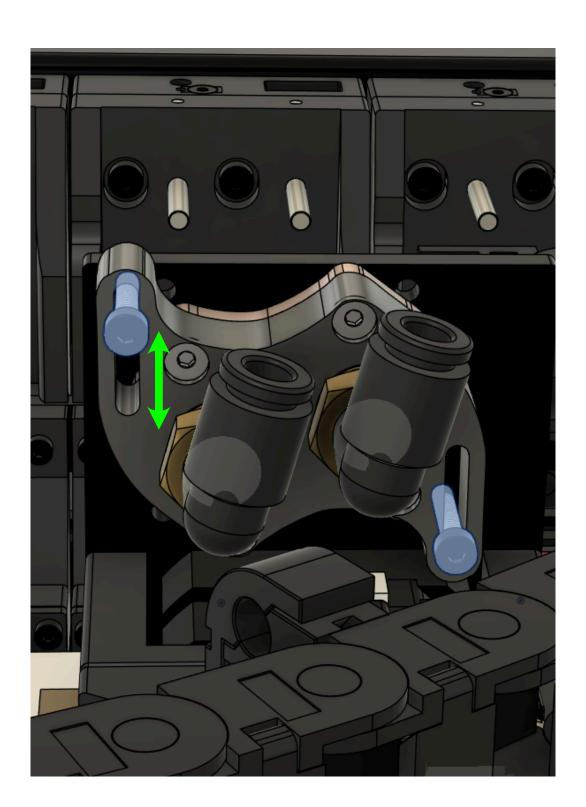
Cut (2) lengths of Nylon Tubing to serve as the plumbing between the left enclosure panel and the previously installed tool head water block. The below render shows these tubes as they installed when fully mounted and secure.
