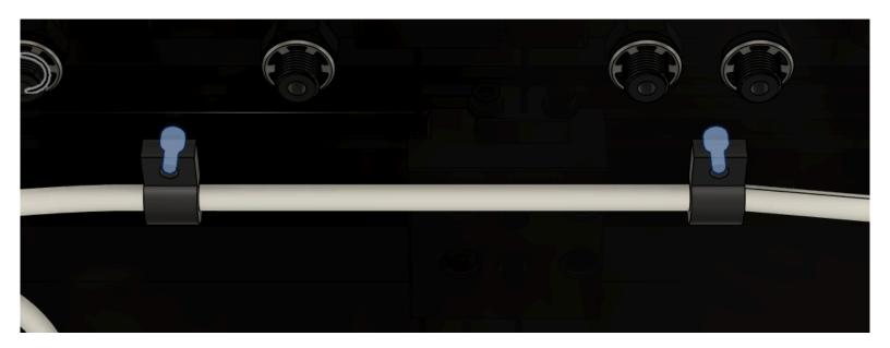
Prepare a length of nylon tubing and install between the water pump and forward tool head tube coupler.
