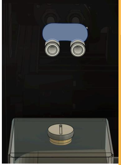
Prepare a length of nylon tubing and install between the conversion fitting and rear-most idle bar coupler.
