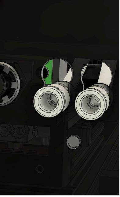
Locate Print\_HosePlug\_Front and insert into the empty space of the keyhole to secure the coupler fittings in place.
