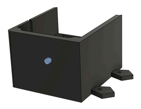
Secure the fan housing to the pump housing using (2) M3x8mm SHCS
