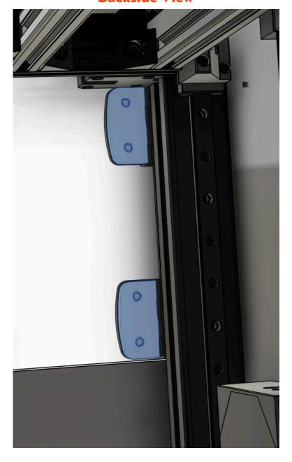
Locate Magnetic\_Latch\_PartB and use (2) M3x8mm FHHS to capture Part B, the door panel and the door handle as shown below.
