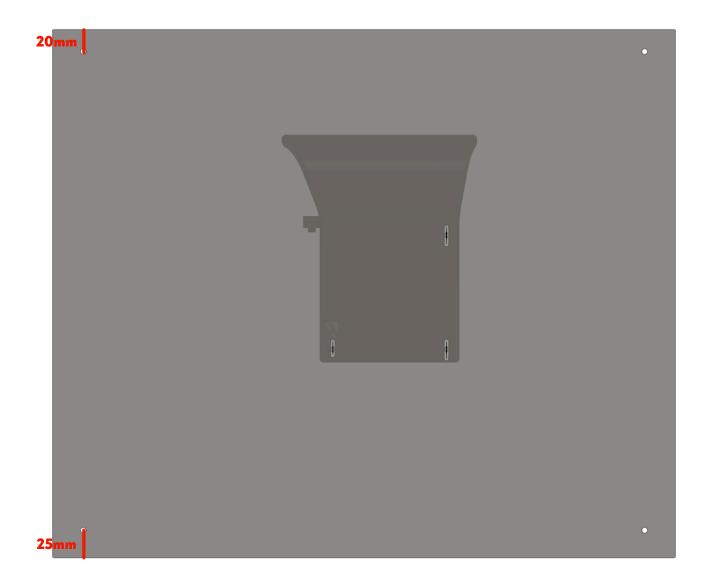
Secure the fan assembly to the acrylic using (3) M4 Thick Fender Washers under (3) M4x20mm SHCS.
