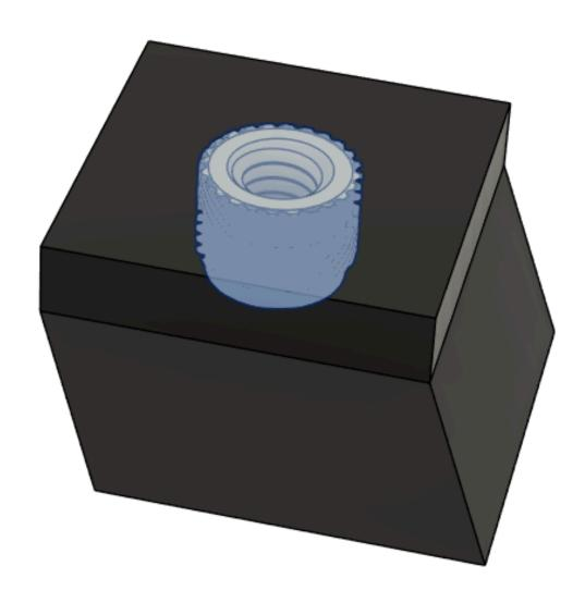
Locate (2) Print\_Door\_Hinge\_Support and install (2) M4 heat set inserts into the location shown. Note the printed part orientation!
