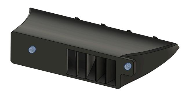
Mate the two previously handled parts as shown below and secure at the outside fastening location using an M4x10mm SHCS
