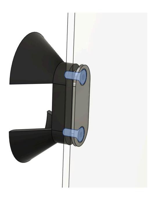
Insert (2) 40 series M4 Tnuts into the rear slot of the left front extrusion as shown.
