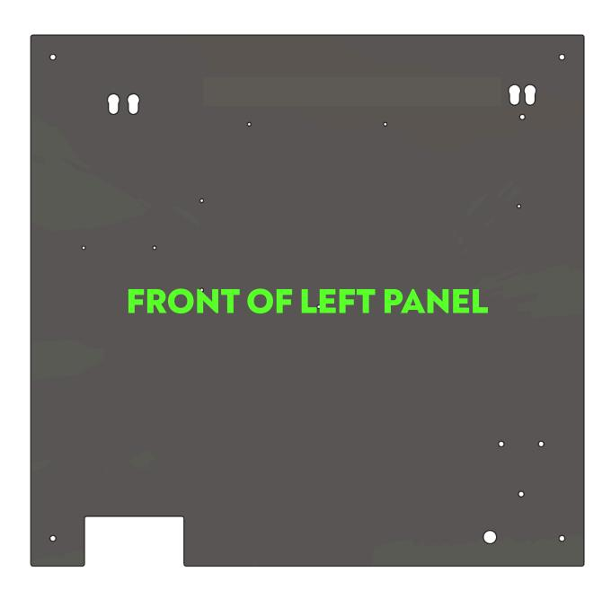
Mount and loosely secure one panel lock at each of the 4 corners of the panel using (4) M4x8mm BHHS. The sharp point of the diamond should face downward, and the head of the fastener will meet the front of the panel. Remember to leave them loose for the time-being!
