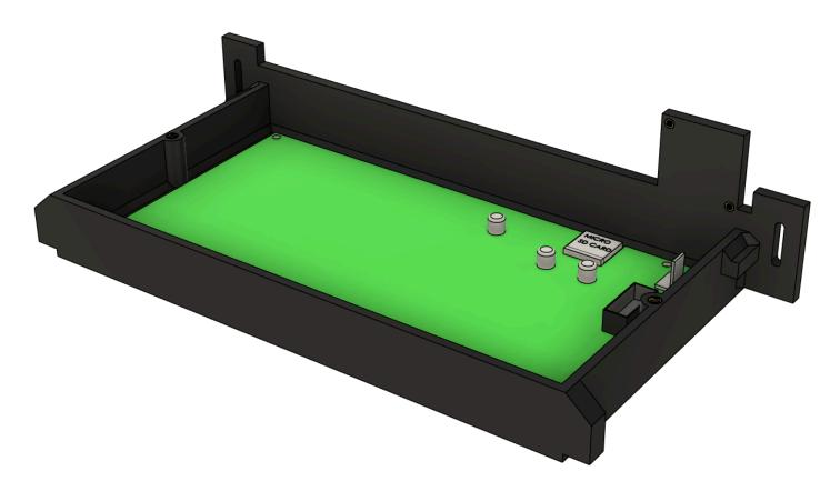
Secure the display to the mount using (4) M3x12 SHCS and (4) M3 Nylon Lock Nuts. Note the direction below!
