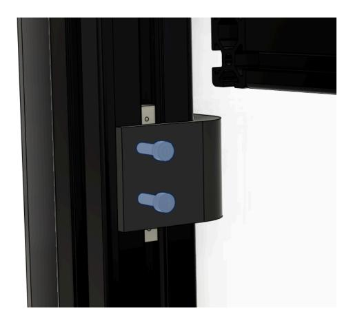
Install the previously assembled latch magnet holder to the mount using (2) M4x8mm FHHS
