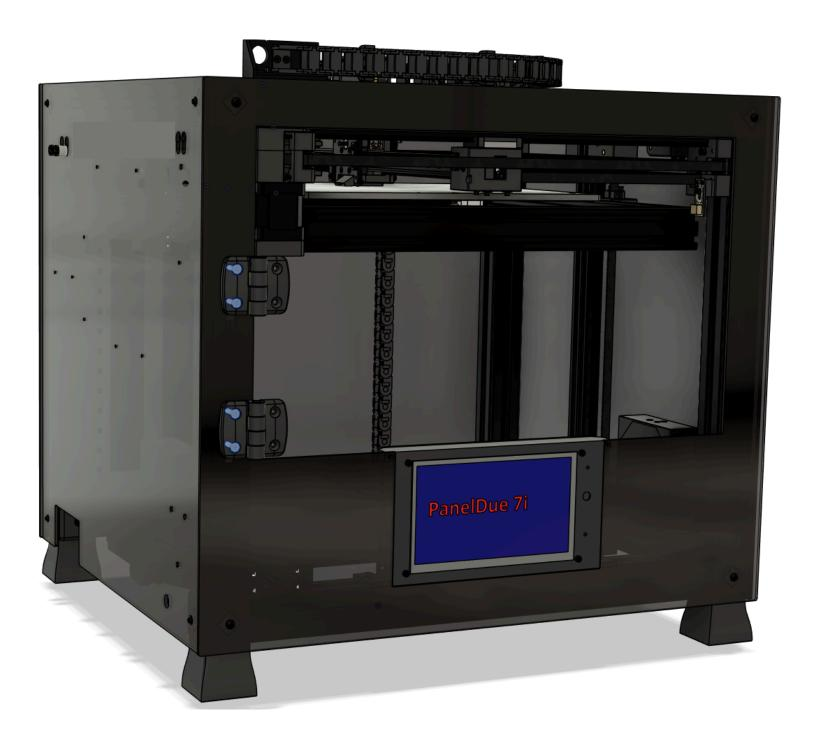
Locate (2) Print\_Door\_Hinge\_Support and use (4) M4x14mm FHHS to capture the open hinge, acrylic door and door hinge supports. Loosely secure these fasteners for now.
