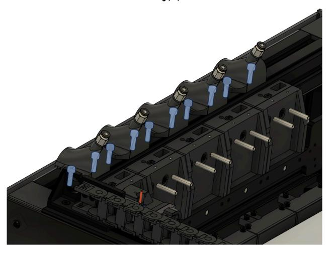
Ensure that the bowen fittings of both the inlet and each FDM tool are roughly in-line
