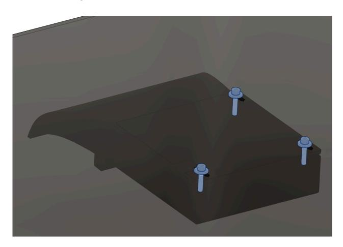
Flip the panel over and install the printed mounts.
