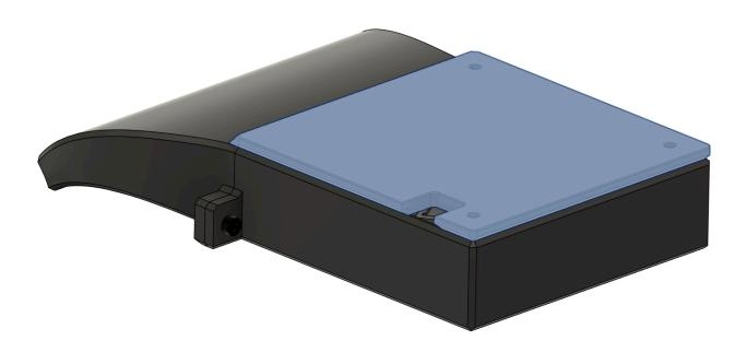
Place the rear acrylic panel over top of the previously assembled fan as shown below. Note the panel orientation for proper fitment!
