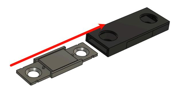
Secure the magnet holder to the magnet mount using (2) M4x8mm FHHS
