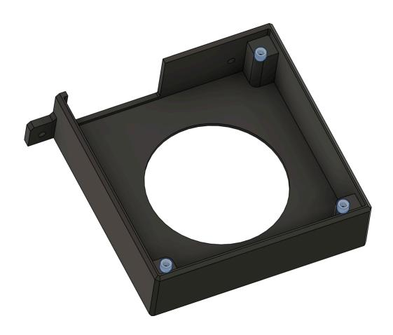
Locate Print\_Aux\_PartCooling\_Duct and install (2) M4 heat set inserts into the shown locations.
