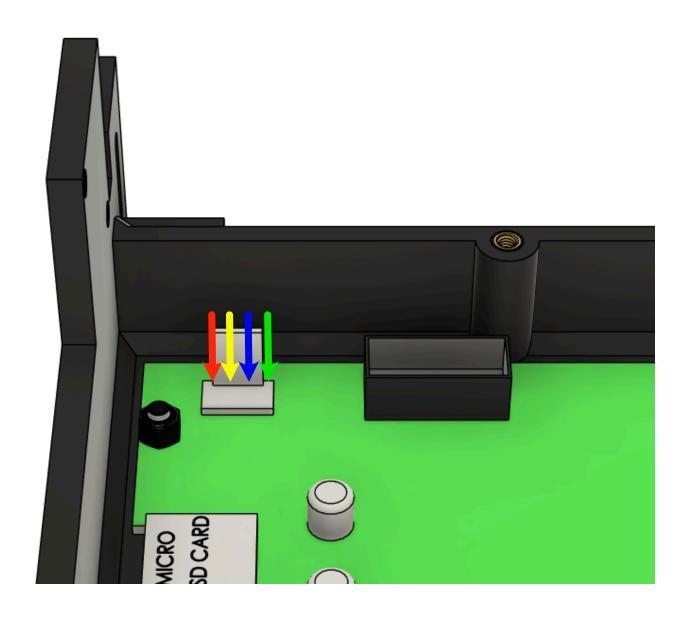
Route the panel due wires to exit the location shown in RED
