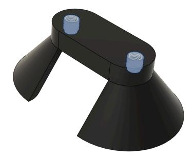
Locate Print\_DoorMagnetMount and install (2) M4 heat set inserts as shown.
