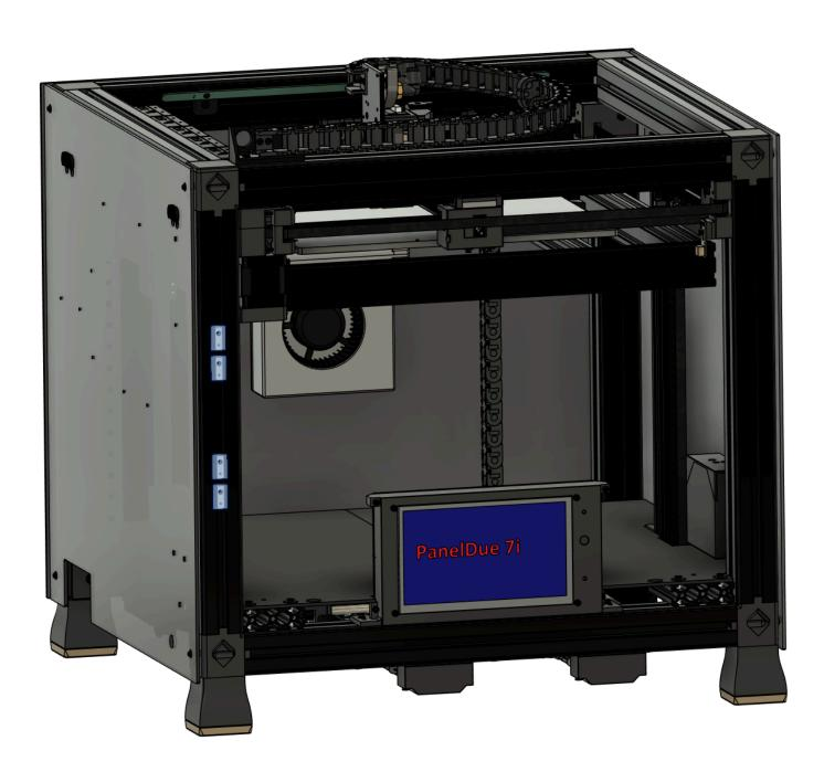
Fit the front panel into place and adjust the position of the installed Tnuts to align with the through holes in the panel
