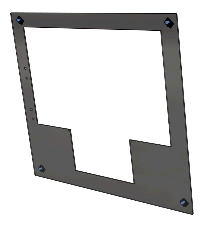
Insert (4) 40 series M4 Tnuts into the outer face of the left front extrusion.
