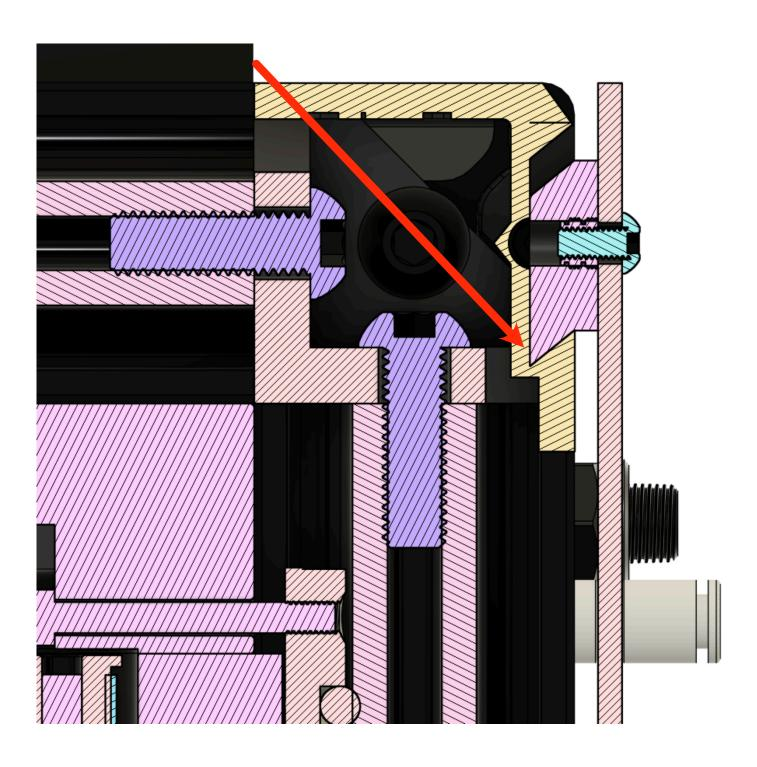
Applying slight inward pressure at the locations shown while tightening the locking lug fasteners can pre-load the panel under light tension - resulting in the best seal.
