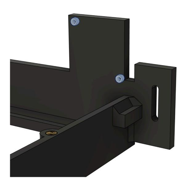
Fit the Panel Due into the housing from the back side of the mount. Note that the fit is meant to be on the tighter side overall. Take care to avoid damage to the LCD ribbon during installation!
