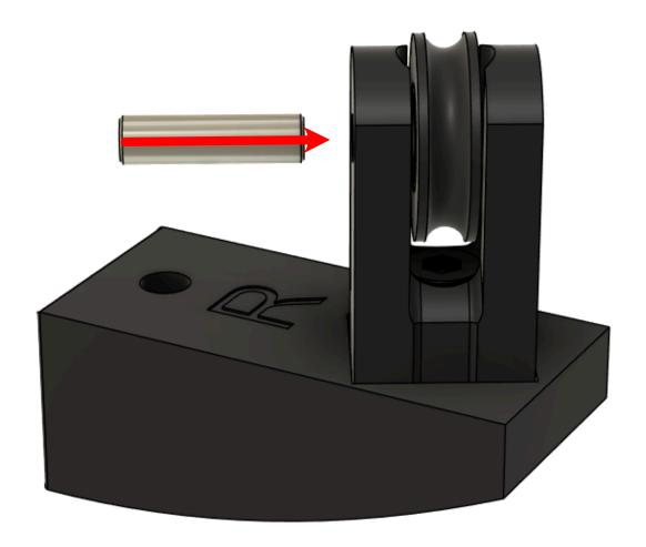
Fit one of each previously assembled Print\_Counterweight\_Lower\_Part 01 to both the left and right dedicated sub assemblies as shown and secure using (2) M4x16mm SHCS.
