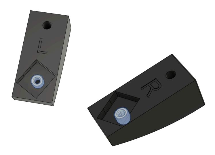
Locate (2) Print\_Counter\_Weight\_Lower\_Part03 and secure to each of the Part02s using an M4x12mm SHCS.
