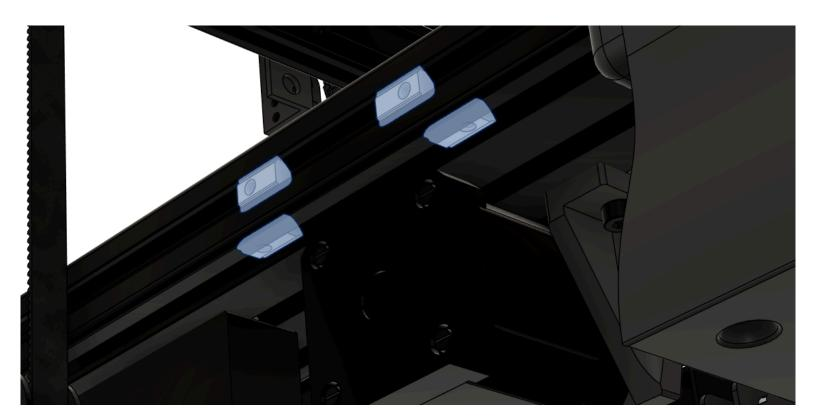
Secure the lower left pulley sub assembly to the extrusion using (2) M4x12mm SHCS in the underside holes.
