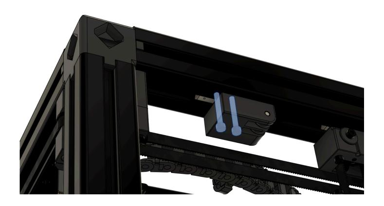
Locate Print\_Counterweight\_Alignment\_Jig\_Upper and fit into the machine as shown below. Slide the upper pulley assembly against the tool face and fully tighten the fasteners.
