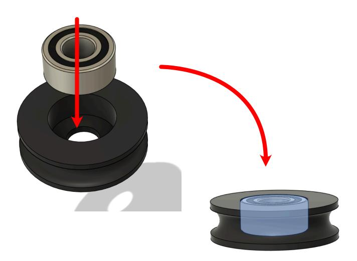
Locate (2) 4x15mm shafts and capture a pulley into each (L + R) lower pulley assemblies.
