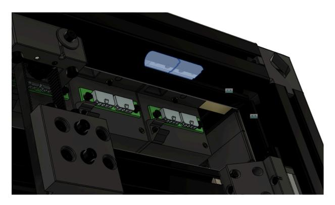
Mount the left side upper counter weight pulley assembly and loosely secure using (2) M4x30mm SHCS.
