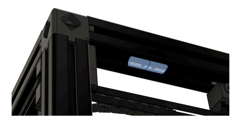
Mount the right side upper counter weight pulley assembly and loosely secure using (2) M4x30mm SHCS.
