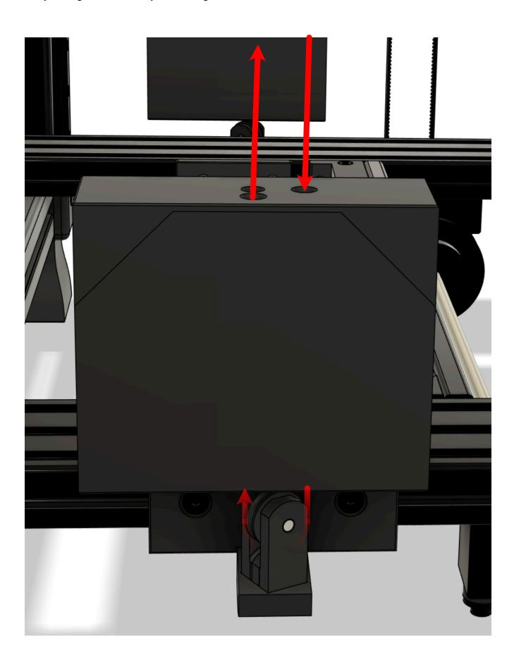
Route the cord upward through the front outer pulley and out toward the rear of the machine
