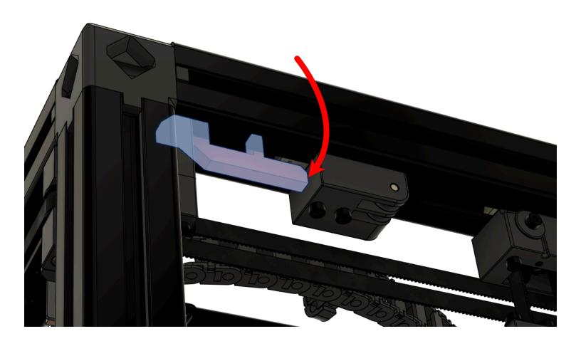
Locate and install (2) 40 series M4 T-nuts and insert both into the forward underside of the top left extrusion as shown.
