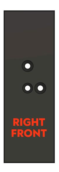
Locate (4) 74mm length 3x5mm PTFE tubes and insert into each of the shown locations (2) on BOTH counter weight containers.
