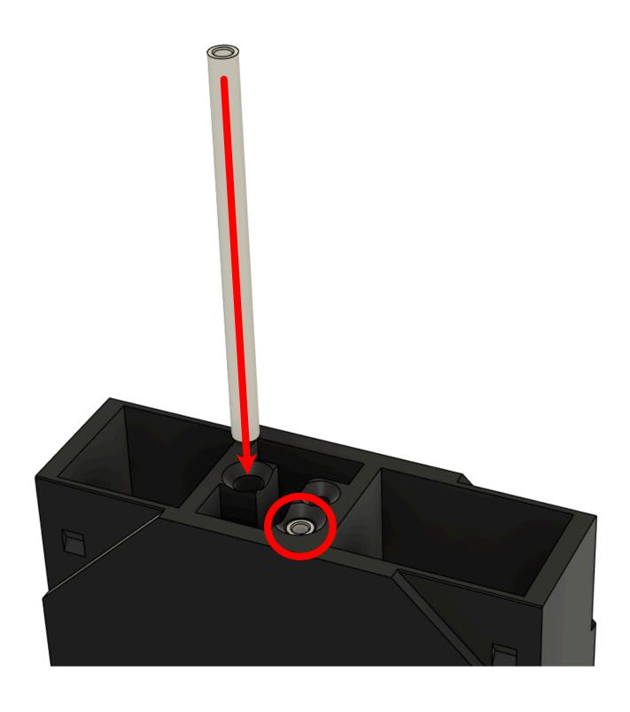
Install the appropriate caps onto each counterweight container.
