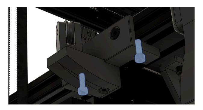
Finish securing with (2) M4x10mm FHHS through the outside facing slot.
