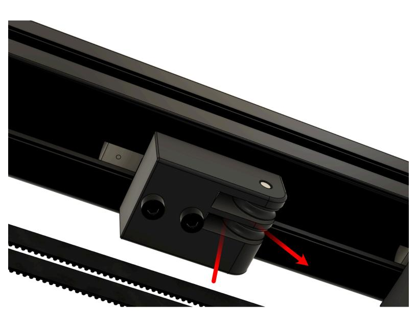
Route the cord downward and through the rearward inside hole of the counterweight container.
