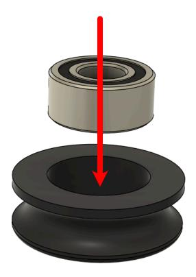
A fully seated bearing will be flush with the top surface of the printed part
