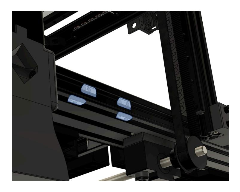
Secure the lower right pulley sub assembly to the extrusion using (2) M4x12mm SHCS in the underside holes.
