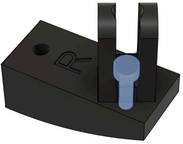
Locate (2) Print\_Counterweight\_Pulley\_Lower and fully seat/install a 4x9x4 ball bearing into each pocket. When fully seated the bearing should be flush with the top face of the printed part.
