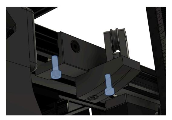
Finish securing with (2) M4x10mm FHHS through the outside facing slot.
