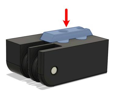
Locate and install (2) 40 series M4 T-nuts and insert both into the forward underside of the top right extrusion as shown.
