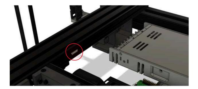
Secure the final 2040 bracket assembly to the 2060 extrusion using the previously inserted 2020 Tnut and (1) M3x8mm BHHS.
