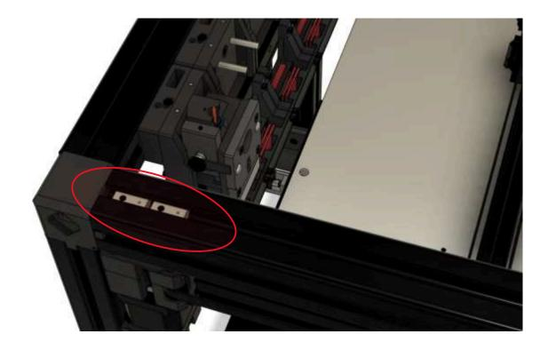
Install and secure the printed part using the previously inserted Tnuts and (2) M4x12mm SHCS. The final installed position should have contact with the edge of the upper corner bracket cover.
