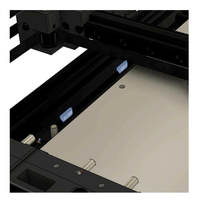
Install and secure the WAGO mount assembly using (2) M4x10mm SHCS. The position of the mount should be roughly centered with the heated bed assembly but is largely non-crucial.
