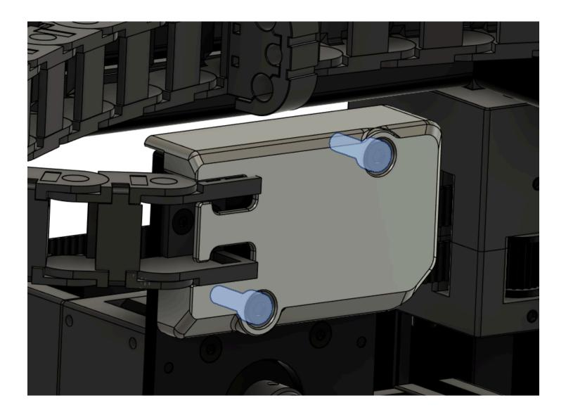
Locate and install the 3010 Blower fan as shown using (2) M2x6mm FHHS.
