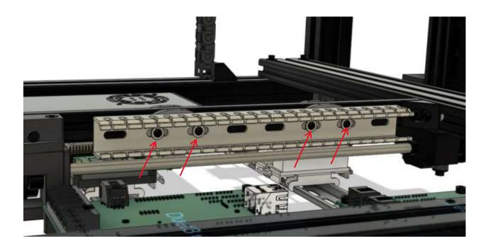
Repeat the above process for the other side of the 2010 extrusion as shown below.
