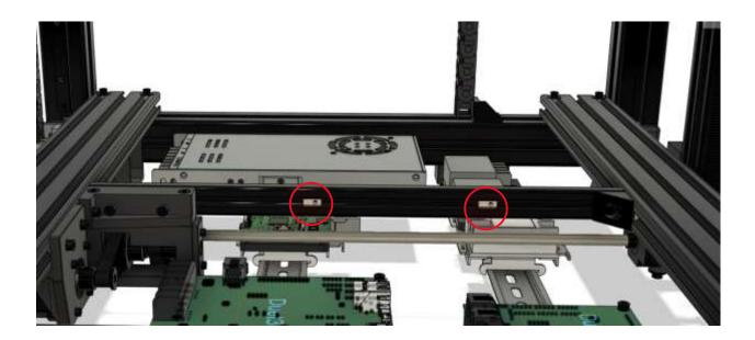
Secure both 2010 bracket assemblies to the 2010 extrusion using the previously inserted 2020 Tnuts and (2) M3x8mm BHHS.
