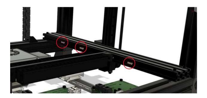
Secure three total 2040 bracket assemblies to the 2060 extrusion using the previously inserted 2020 Tnuts and (3) M3x8mm BHHS.
