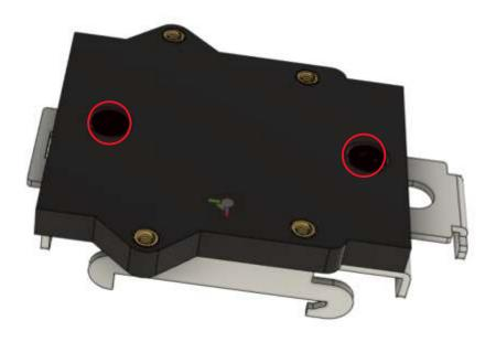
Secure one of two DC converters to the printed part using (4) M3x6mm SHCS.
