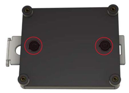
Secure the Pi to the printed part using (4) M2x8mm SHCS.
