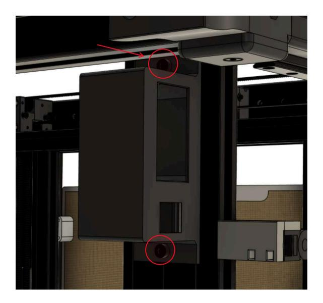
Install the CAT6 keystone jack into the housing as shown below. This is also the location for the Power Inlet/AC switch combination part. It is recommended to first pre-wire the AC switch before installation. Please see the CE wiring guide or leave the AC switch dismounted for now.
