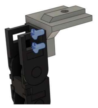
Secure the other end of the drag chain to the previously installed chain mount assembly using (2) additional M3x6 FHHS as shown below:
