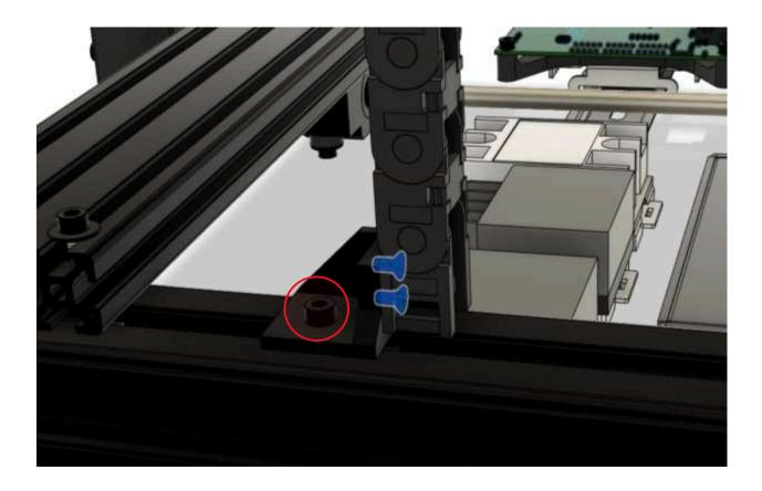
Slide the loosely mounted lower assembly as needed to achieve a parallel path for both vertical portions of the Z drag chain as shown below. Fully tighten in this position.
