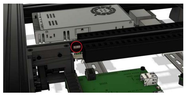
Locate Print\_Wire\_Duct\_Shield and secure to the 2010 extrusion using the previously inserted Tnut and (1) M3x8 BHHS as shown below:
