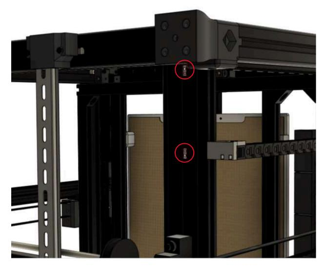
Install (2) 2020 M4 Tnuts into the bottom center slot of the 2060 extrusion as shown below:
