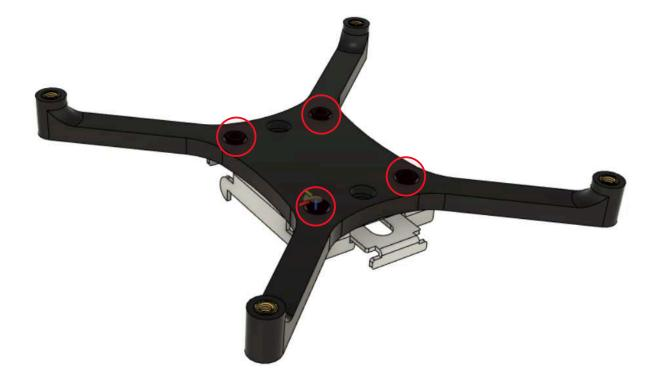
Secure the Duet 3 6HC Main Board to the assembly using (4) M4x6mm SHCS. Note the orientation of the board during installation.
