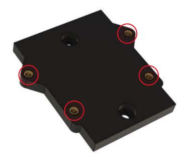
Locate Print\_DCConverter\_Mount and install (4) M3 heat set inserts at the shown locations.
