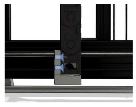
Loosely install the upper chain mount using the previously inserted 4040 Tnut and (1) M4x12mm SHCS.
