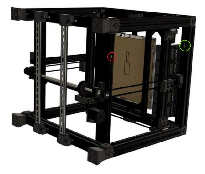
Locate Print\_Jig\_StaticChainLower and position as shown below to ensure that the lower static chain assembly is properly spaced along the 2060 extrusion. Secure the lower static chain mount assembly using (1) M4x10 SHCS into the previously inserted 2020 Tnut.
