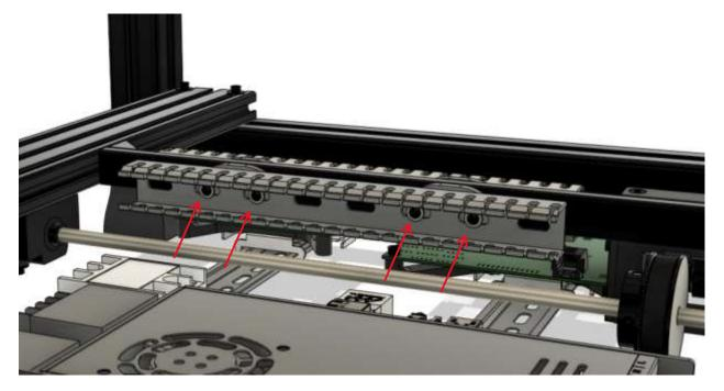
Insert an additional 2020 M3 Tnut into the 2010 extrusion in the shown location:
