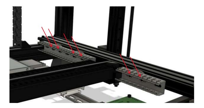
Insert (1) 2020 M3 Tnut into the inside facing slot of the left 2060 extrusion as shown below:
