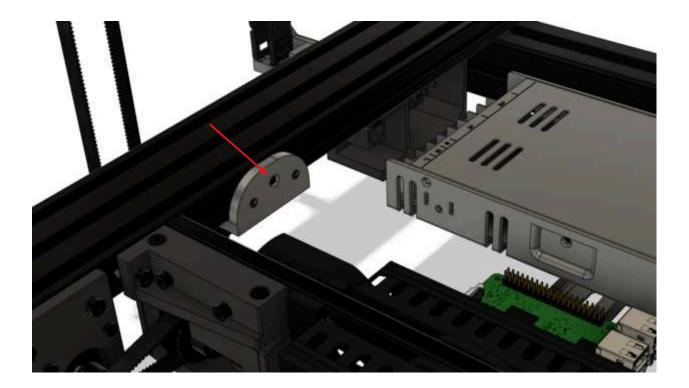
Locate (1) 100mm length of 25mmx25mm cable duct. Remove the cover and secure the main body to the forward-facing surface of the 2040 duct mount assembly. This requires (2) M3 fender washers and (2) M3x6mm BHHS.
