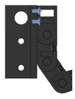
Locate Print\_ZChainMount\_Top and install (2) M3x4.6x4 heat set inserts into the locations shown below.
