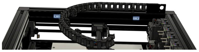
Install both LED Light Bar assemblies using (4) total M4x12mm SHCS at all mounting point locations. The LED Bars should be roughly centered within it's length of extrusion.
