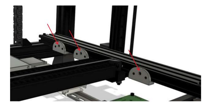
Locate (1) 200mm length and (1) 100mm length of 25mmx25mm cable duct. Remove the cover and secure the main body to each of the forward-facing surfaces of the 2040 duct mount assemblies. This requires (6) M3 fender washers and (6) M3x6mm BHHS. Note that the 200mm duct is installed rearward of the Z axis drive 2010 extrusion.
