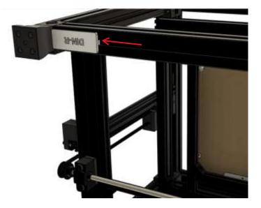
Attach one of the DIN Rail Assemblies to the machine frame using (4) M4x30mm SHCS as shown in red below. Be sure to tighten into place against the printed jig. Confirm the DIN rail is square with the machine by moving the printed jig to the other side as well! Perfect squareness is not critical.
