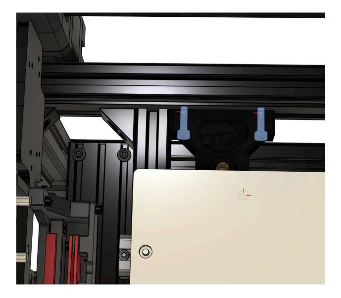
Drop (1) 5x43mm bearing steel shaft down into the part through the sleeve bearings and confirm that a light press audibly activates the micro switch. Note that this shaft is not secured and may fall out if the machine is overturned at any time.
