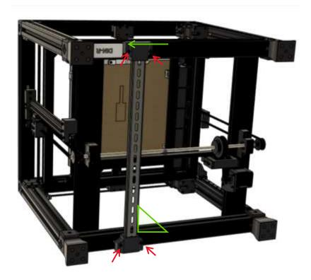
Remove the printed tool and set aside. Repeat the above procedure for the second DIN rail assembly but this time using Print\_Jig\_DINSpacerCenter to set the distance between the first and second DIN rail assembly as shown below.
