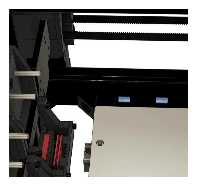
Install Sex Bolt sub assembly and secure using (2) M4x14 SHCS. The installed location of the assembly should be such that the printed part is flush with the 2020 extrusion itself. This position can be adjusted in firmware later if needed.
