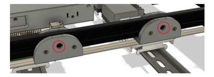
Locate a 230mm length of 25mmx25mm cable duct. Remove the cover and secure the main body to each of the forward-facing surfaces of the 2010 duct mount assemblies. This requires (4) M3 fender washers and (4) M3x6mm BHHS.
