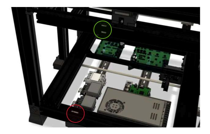
Loosely attach the upper Z chain mount with drag chain to the previously inserted 2020 Tnuts using (2) M4x8mm SHCS shown below in red. Locate Print\_Z\_Chain\_Mount\_Top\_Installation\_Tool (shown in blue below) and use it set the location of the z chain mount. Fully tighten the fasteners once this location is achieved.
