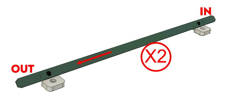
Insert (2) 40 Series M4 T-nuts into each of the inside extrusion extrusion slots of the top most part of the frame. Use (4) total T-nuts to populate the front and rear extrusions.
