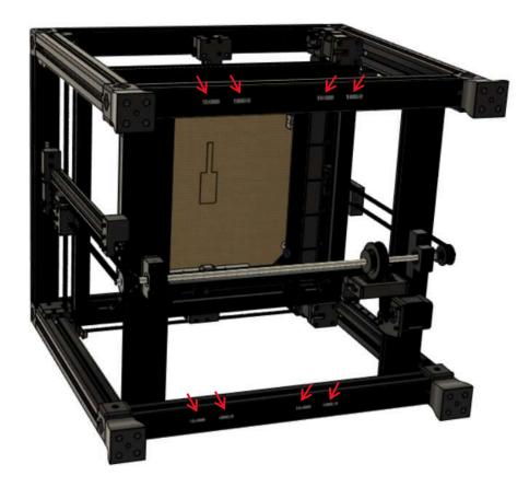
Locate Print\_Jig\_DINSpacerRight and place into the upper left extrusion as viewed from the angle below. Seat against the face of the machine foot.
