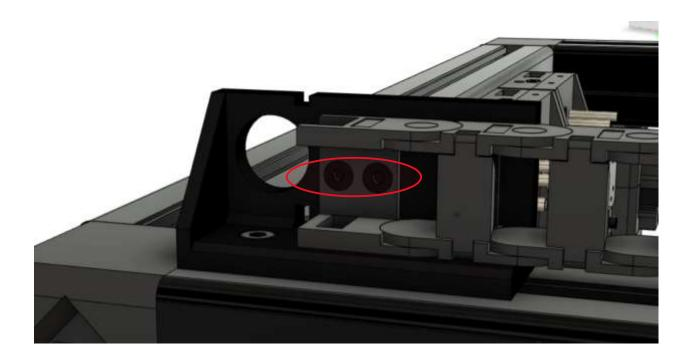
Secure the other end of the XY chain to the upper left face of the X-Plate using (2) M3x6mm FHHS as shown below.
