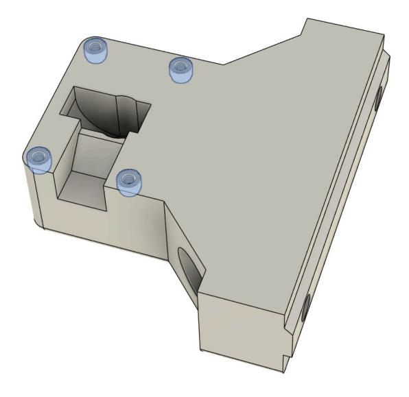
Insert (2) 5x7x8mm copper sleeve bearings from the top. There is a seat in the printed housing to prevent them from going too far.
