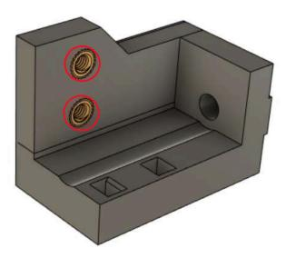
Locate Print\_ZChainMount\_Bottom and repeat the above with an additional (2) heat set inserts at the shown locations:
