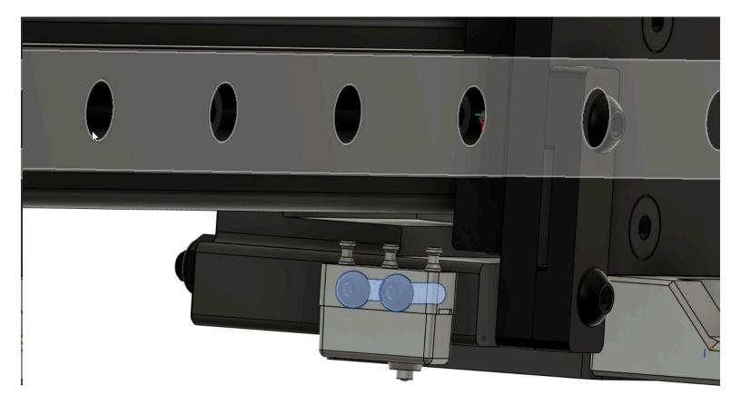
Locate and install Print\_ToolHead\_Wire\_Cover as shown below using (2) M4x12mm SHCS.
