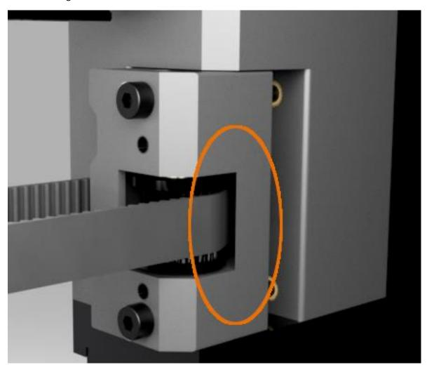
Route the loose end of the XY belt through the rear XY corner bracket around the lower pulley and through the slot towards the front. Again, the toothed face of the belt is to mate with the toothed pulley profile.
