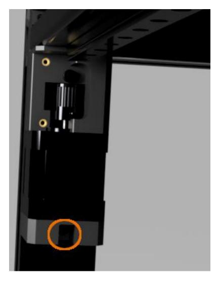
Locate Print\_XY-Axis\_Motor\_Bracket\_Front\_Part05 and tap M3 threads into the specified hole below.
