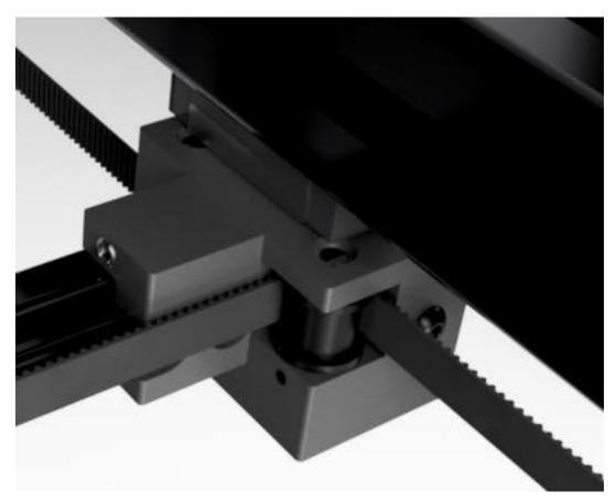
Now route the loose end of this XY belt through the front XY motor assembly. The toothed face of the belt faces the toothed pulleys. Start by feeding the belt around the motor pulley and having the belt exit the motor assembly through the tensioner idler.
