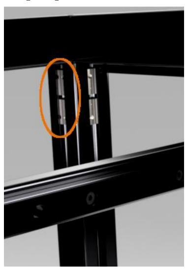
Locate Print\_XY-Axis\_BlackStop\_Mount and install a M3\_4.6x4mm\_Heat\_Set\_Insert into the location shown below.
