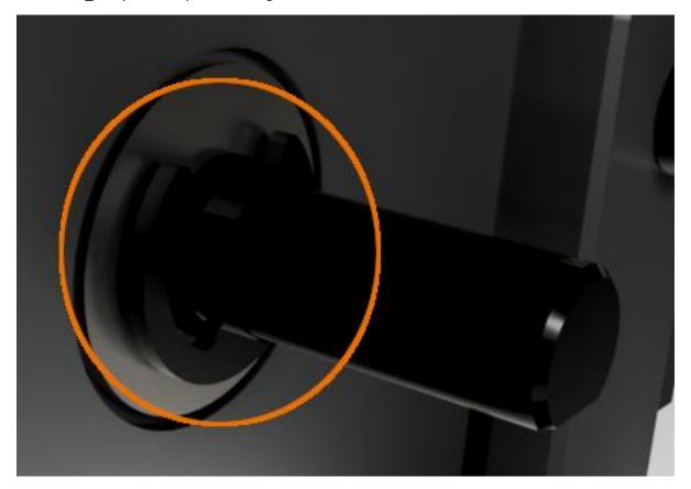
Slide three more T-Lock\_Shim onto the end of the T-lock and slide them all the way to the E-Clip.
