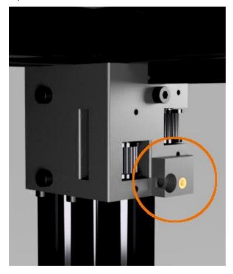
Install a DIN912\_M4\_30mm\_SHCS into the location shown below and fully tighten.
