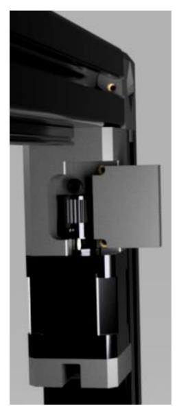
Place the tensioner assembly onto the motor housing and secure it to the housing with two M3\_35mm\_BHHS. Tighten the screws equally until the pre-tensioning tool has some drag when moved. It is more important to try and keep the tensioner parallel to the motor housing than to have the position exact. The final position of the tensioner will occur later during the belt tensioning process.
