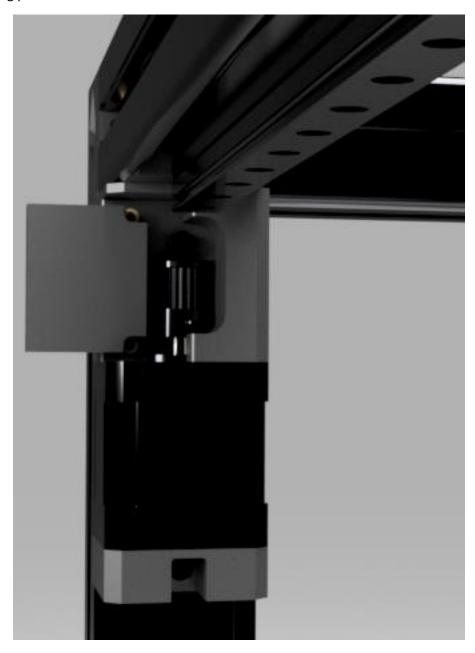
Place the tensioner assembly onto the motor housing and secure it to the housing with two M3\_35mm\_BHHS. Tighten the screws equally until the pre-tensioning tool has some drag when moved. It is more important to try and keep the tensioner parallel to the motor housing than to have the position exact. The final position of the tensioner will occur later during the belt tensioning process.
