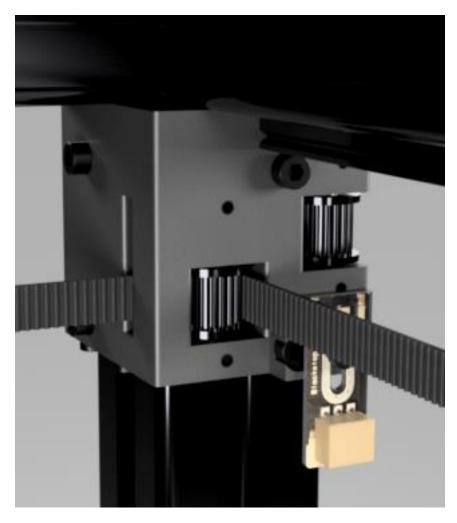
Route the loose end of the XY belt through the front Y-Axis bracket around the toothed pulley and toward the X-Plate.
