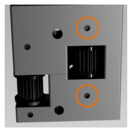
With the hand vise still clamping the corner bracket assembly together, install two DIN912\_M3\_25mm\_SHCS in the locations below and fully tighten.
