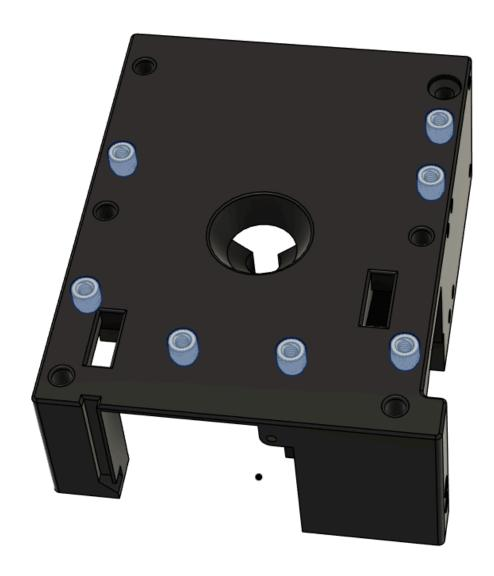
Rotate the printed part and install two M3\_4.6x4mm\_Heat\_Set\_Insert into the locations shown below.
