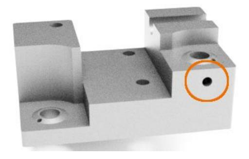
Now locate the Print\_Y-Axis\_Bracket\_Rear\_Top\_(1.52mm) and tap the specified hole below with M3 threads.
