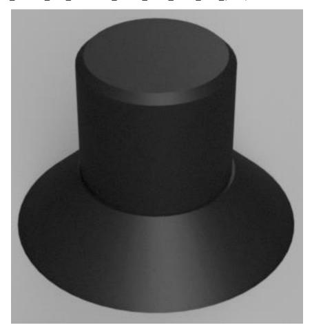
Press one printed installation tool into the top and bottom of the tensioner assembly.
