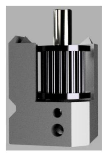
Press Print\_XY-Axis\_Motor\_Bracket\_Rear\_Part06 on to the tensioner assembly as shown below.
