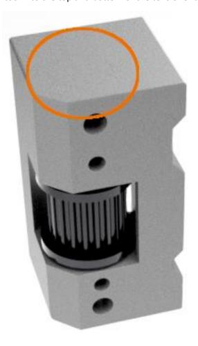
Using your hand vise, compress the two halves of the belt tensioner assembly setting the position of the linear shaft. Install two DIN916\_M3\_5mm\_Set\_Screw into the locations shown below and fully tighten.
