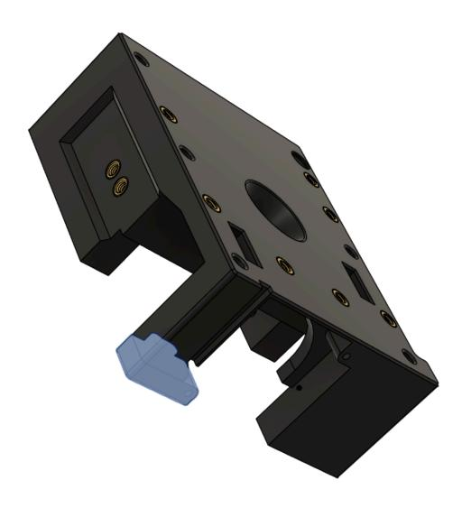
Line up the X-Bracket assembly to the back of the X-Plate and loosely secure with a DIN912\_M3\_35mm\_SHCS as shown below.
