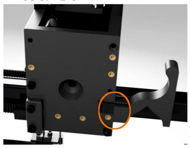
Locate Print\_BeltClamp\_Right\_Rear and loosely secure with a DIN912\_M3\_40mm\_SHCS. Note:Orient this printed part so the edge of the printed clamp is flush with the rear edge of the X-Bracket.
