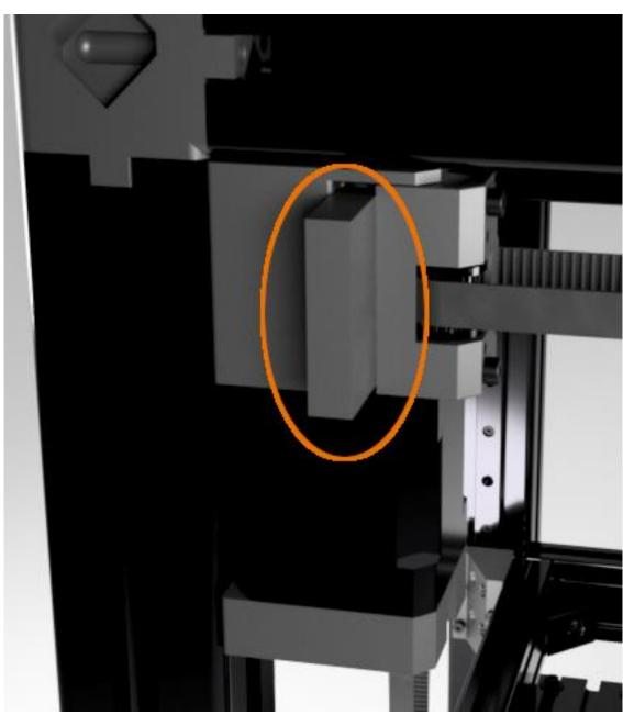
This is a good time to verify that the tensioner block is parallel to the motor housing. Adjust the screws to keep the tensioner flush to the pre-tensioning tool. Attach a belt puller tool to end of the XY belt you are adjusting. We will only remove slack from the printed side of the X-Carriage assembly by loosening the printed belt clamps. Be certain to attach the belt puller to the proper belt end.
