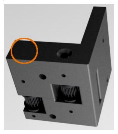
Using your hand vise, compress the two halves of the corner bracket assembly setting the position of the linear shaft. Install two DIN916\_M3\_5mm\_Set\_Screw into the locations shown below and fully tighten.
