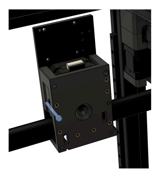
Install one end of  $GT2_894t_Belt_9x1788mm_(1.52mm)$  through the back of the X-Plate with belt teeth oriented as shown below.
