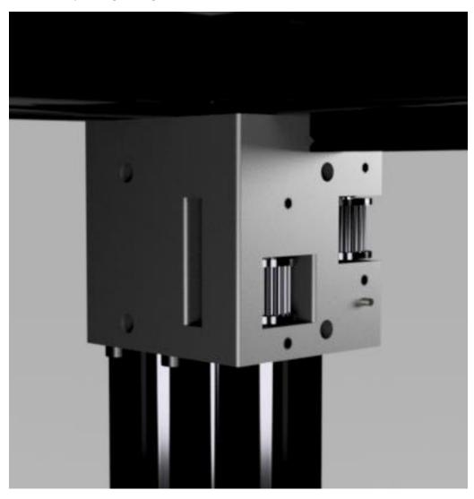
Install two DIN912\_M4\_20mm\_SHCS into the locations shown below and fully tighten.
