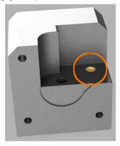
Locate Print\_XY-Axis\_Motor\_Bracket\_Rear\_Part02\_CE and install a M3\_4.6x4mm\_Heat\_Set\_Insert in the position shown below.
