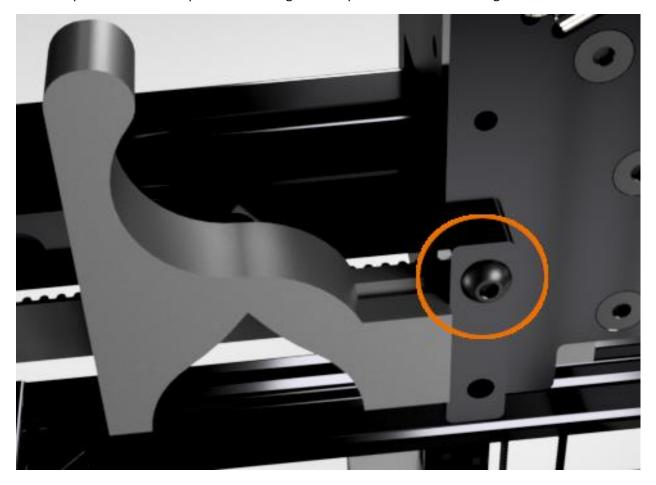
Insert a ISO7380\_M3\_45mm\_BHHS fully into the location shown below.
