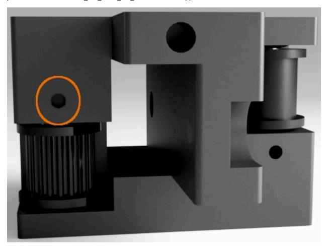
Remove the hand vise and the linear rail installation tools. Move the linear installation tools to the corresponding positions of the other linear rail in the bracket assembly.
