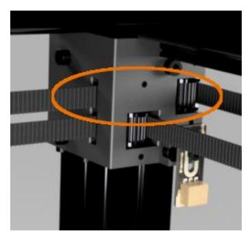
Continue to route the loose end of the XY belt through the rear XY corner bracket slot then around the upper pulley and out toward the left.
