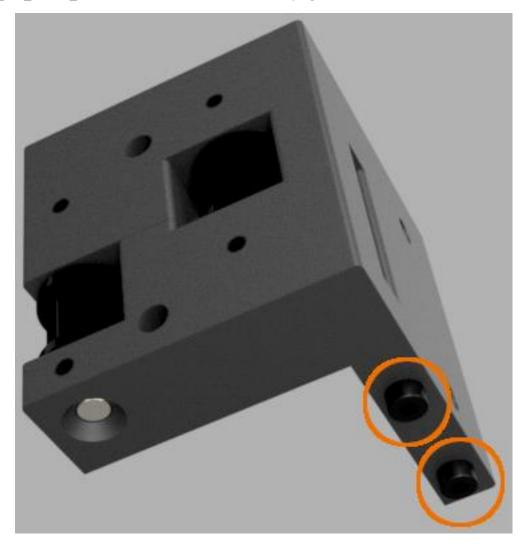
Remove the hand vise and the printed installation tools. Install two Tnut\_40Series\_M4 into the top of the rear right extrusion as shown.
