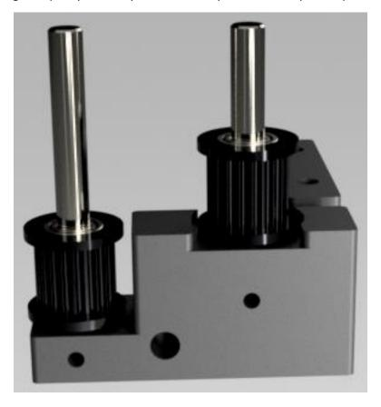
Press the Print\_XY-Axis\_Belt\_Corner\_Bracket\_Rear\_Top onto the corner bracket assembly.
