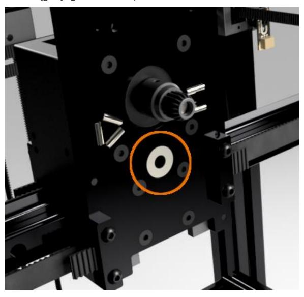
$Locate\ Print\_Bearing\_Flanged\_Pocket\_5x10x4mm\ and\ snap\ into\ back\ of\ X-Bracket\ as\ shown.$
