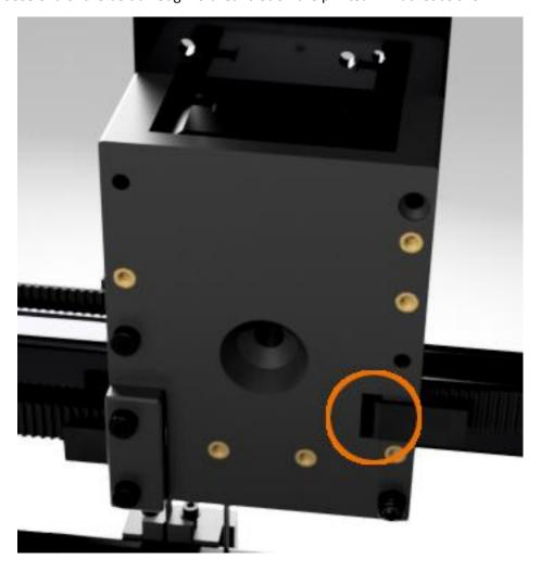
Attach a Print\_XY\_Belt\_Tightening\_Tool\_(1.52mm) to the end of XY belt.
