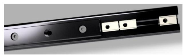
Slide the assembled Y-Axis Bracket Front onto the X-Axis linear rail assembly and line the holes in the roll-in nuts with the holes in the printed assembly.
