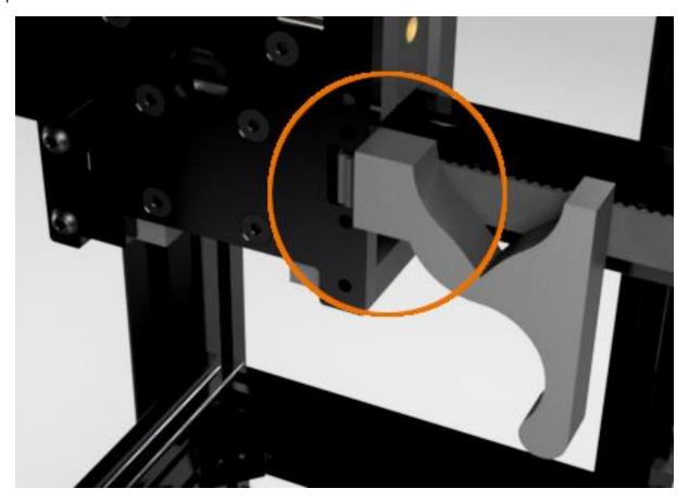
Locate the remaining CNC\_Belt\_Clamp\_Left and loosely attach to the X-Plate with two ISO7380\_M3\_8mm\_BHHS as shown.
