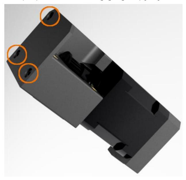
Place two Tnut\_40Series\_M4 into the front left extrusion of the frame as shown below.
