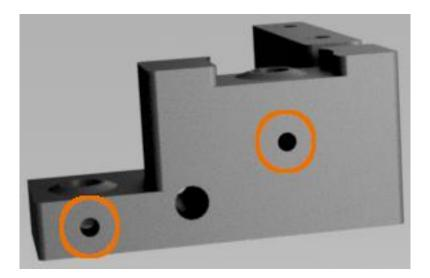
Locate Print\_XY-Axis\_Belt\_Corner\_Bracket\_Rear\_Top and tap M3 threads into the two hole locations shown below.
