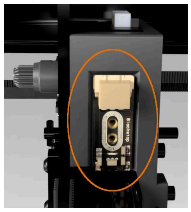
Secure the BlackStop to the X-Bracket with two DIN912\_M3\_6mm\_SHCS.
