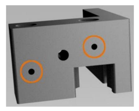
Return to Print\_XY-Axis\_Belt\_Corner\_Bracket\_Front\_Top and install two M3\_4.6x4mm\_Heat\_Set\_Insert into the locations shown below.
