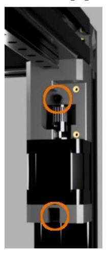
Locate Print\_XY-Axis\_Motor\_Bracket\_Front\_Part05 and tap M3 threads into the specified hole below.
