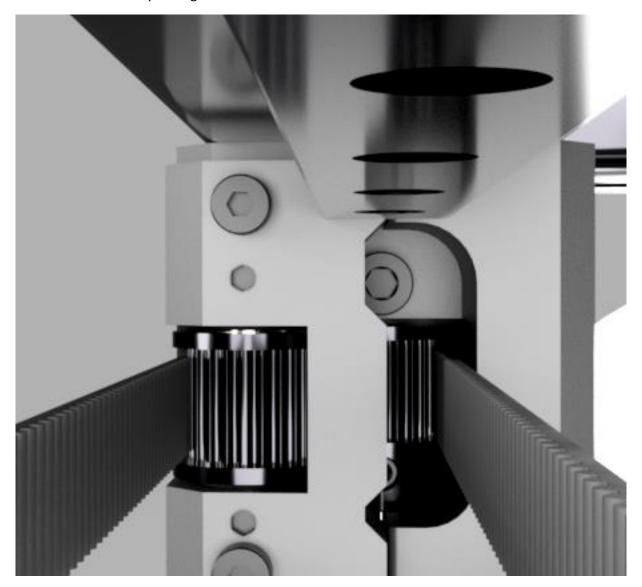
The toothed belt should only come in contact with the toothed pulleys. It should not rub or touch any other part of the machine. Verify that belt is going through tensioner housing and not around the tensioner housing.
