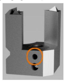
Locate Print\_XY-Axis\_Motor\_Bracket\_Rear\_Part06 and tap M3 threads into the specified hole below.
