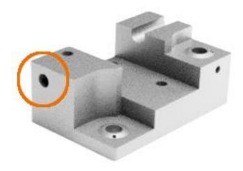
Return to the Print\_Y-Axis\_Bracket\_Front\_Top\_(1.52mm) and tap the specified hole below with M5x0.5 threads.
