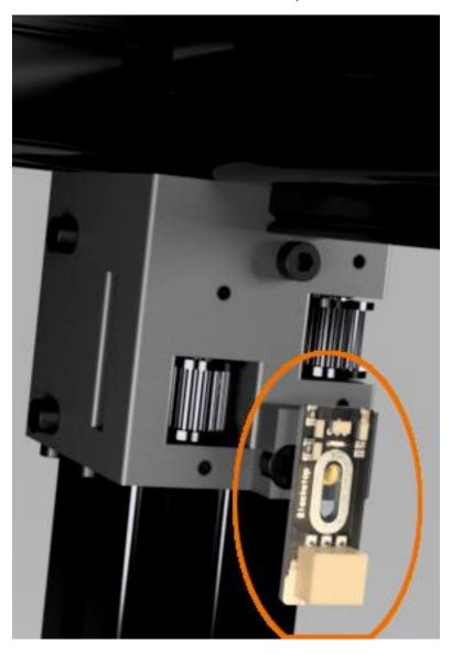
Install a DIN912\_M3\_8mm\_SHCS to secure the BlackStop as shown.
