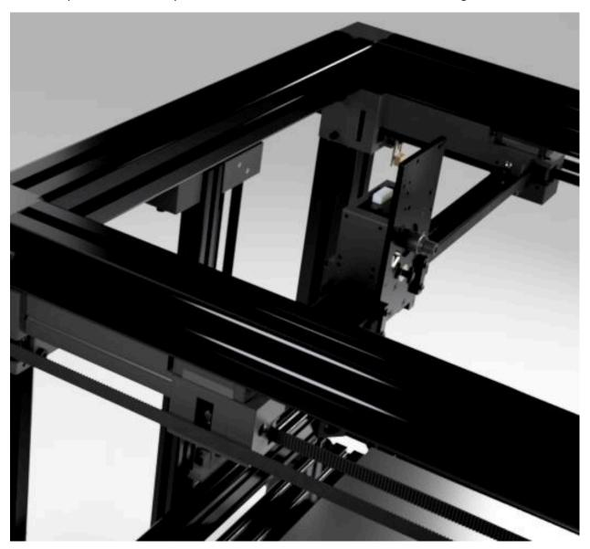
The goal is to tighten the tension in each of the XY belts as to prevent skipped steps during operation. Contrary to popular belief, excessively tight belts are not better. Excessive belt tension adds to vibration in the X-Gantry that leads to surface defects on the print. In the tuning guide, input shaping calibration will reveal if the belts are too tight. We will begin by equally tightening the screws on one of the XY belt tensioners.
