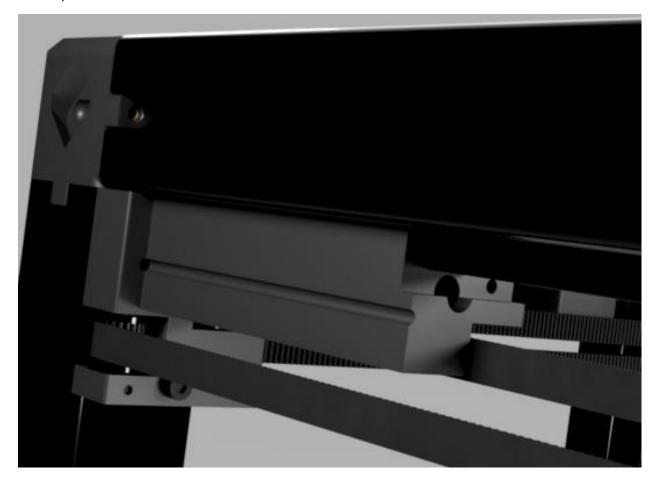
Now slowly move the X-Gantry until both Y-Axis brackets are flush to the tensioning tools.
