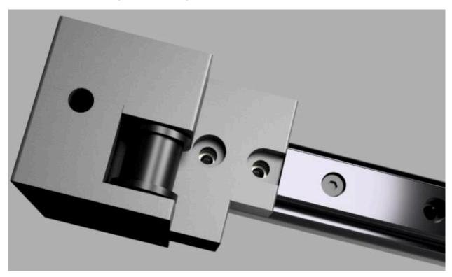
Install two DIN912\_M4\_10mm\_SHCS into the locations shown below and fully tighten.
