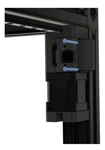
Remove the printed pre-tensioning tool.
