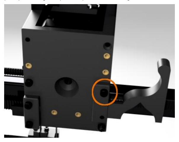
Loosely secure the other end of the printed clamp with a DIN912\_M3\_10mm\_SHCS.
