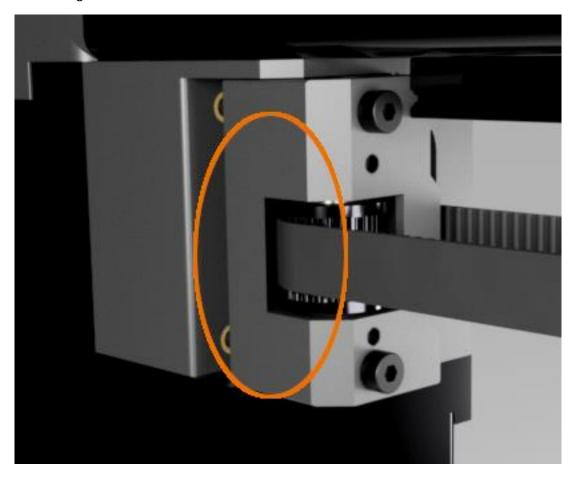
Route the loose end of the XY belt through the front XY corner bracket around the upper pulley and through the slot towards the rear. Again, the toothed face of the belt is to mate with the toothed pulley profile.
