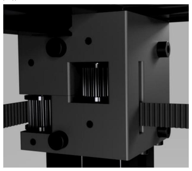
Continue to route the loose end of the XY belt through the front XY corner bracket slot then around the lower pulley and out toward the left.
