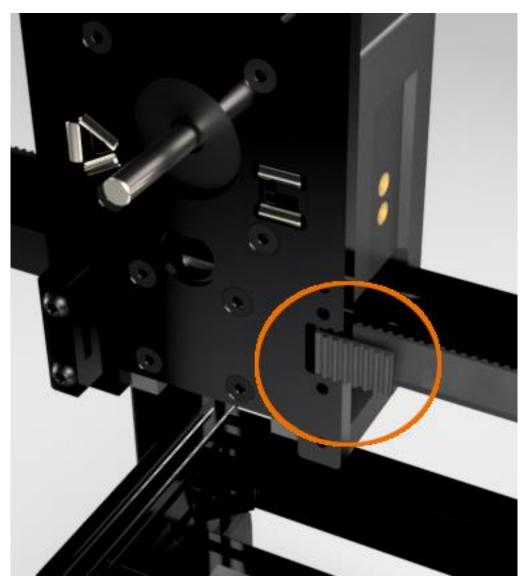
Attach the Print\_XY\_Belt\_Tightening\_Tool\_(1.52mm) to the end of the XY belt as shown. Note:The printed tool is inverted when installed on this side of the X-Plate.
