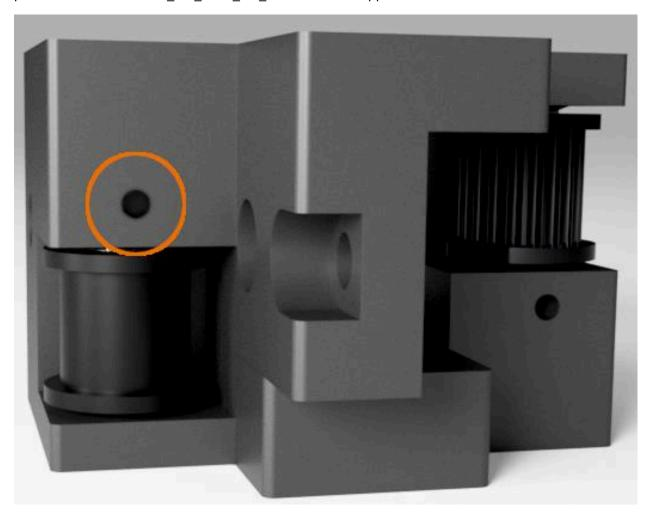
Remove the hand vise and the linear rail installation tools. Move the linear installation tools to the corresponding positions of the other linear rail in the bracket assembly.
