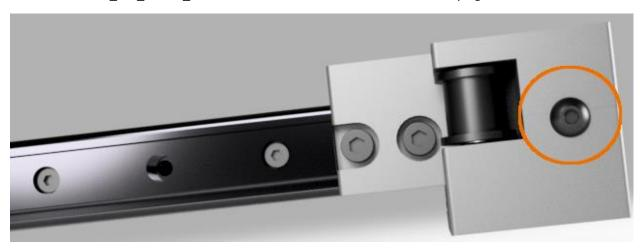
Position the assembled X-Gantry inside of the machine frame with the linear rail facing the left side of the machine. Remove the blue painters tape from the MGN-12 linear rail cartridge of the front Y-Axis rail (if previously installed) and line it up to the front Y-Axis bracket of the X-Gantry. Secure the bracket to the gantry with three M3 Fender washers and three DIN912\_M3\_40mm\_SHCS.
