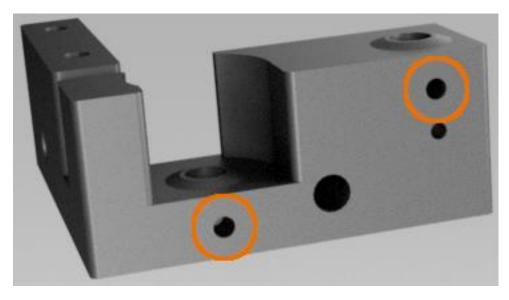
Locate Print\_XY-Axis\_Belt\_Corner\_Bracket\_Front\_Top and tap M3 threads into the two hole locations shown below.
