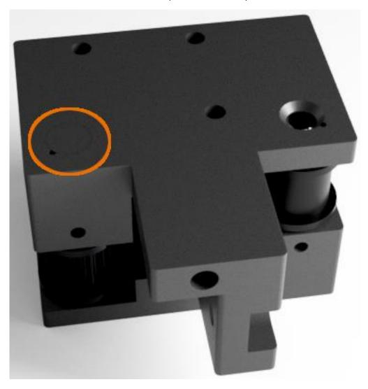
Place the other tool into the recess on the bottom of the bracket assembly and then use your hand vise to clamp the two halves of the bracket assembly together setting the shaft in the proper centered position. Install a DIN916\_M3\_5mm\_Set\_Screw into the tapped hole as shown below.
