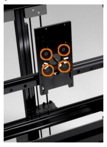
Locate Print\_X\_Bracket\_V2\_Part\_1 and install seven M3\_4.6x4mm\_Heat\_Set\_Insert into the locations shown below.
