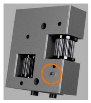
Install two Tnut\_40Series\_M4 into the top of the front right extrusion as shown.
