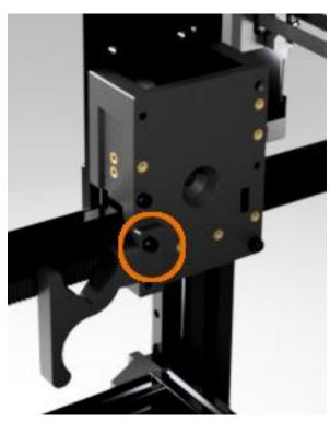
Loosely secure the other end of the printed clamp with a DIN912\_M3\_40mm\_SHCS.
