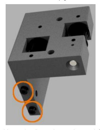
Remove the hand vise and the printed installation tools. Locate the Linear\_Shaft\_2x6mm. Press the linear shaft into the location shown below until fully seated.
