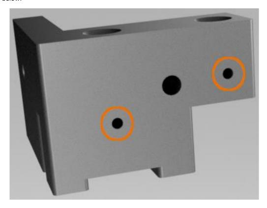
Locate Print\_XY-Axis\_Belt\_Corner\_Bracket\_Rear\_Bottom and tap M3 threads into the two hole locations shown below.
