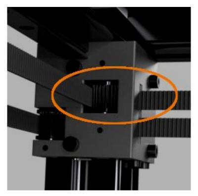
Route the loose end of the XY belt through the rear Y-Axis bracket around the toothed pulley and toward the X-Plate.
