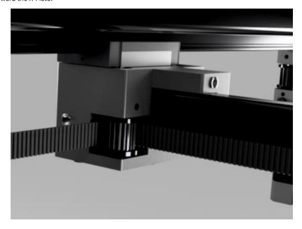
Route the loose end of the belt through left front slot on the printed X-Bracket as shown.
