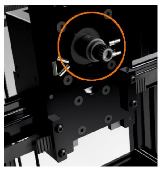
Secure the extruder drive gear to the shaft with a DIN916\_M3\_4mm\_Set\_Screw. As this screw tightens, wiggle the extruder gear to assure the flat end of the set screw mates flush with the flat of the NEMA 17 motor shaft. Keep the hub of the extruder gear slightly above the face of the motor to prevent the gear from rubbing against the motor while turning. Tighten the M3x4mm set screw completely.
