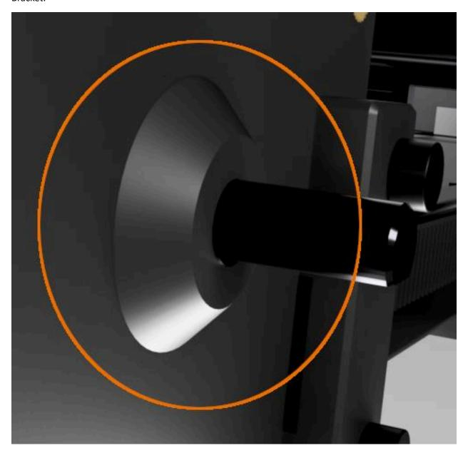
Locate a BlackStop and place on the front of the X-Bracket as shown.
