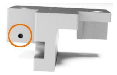
Now locate the Print\_Y-Axis\_Bracket\_Front\_Top\_(1.52mm) and tap the specified hole below with M3 threads.
