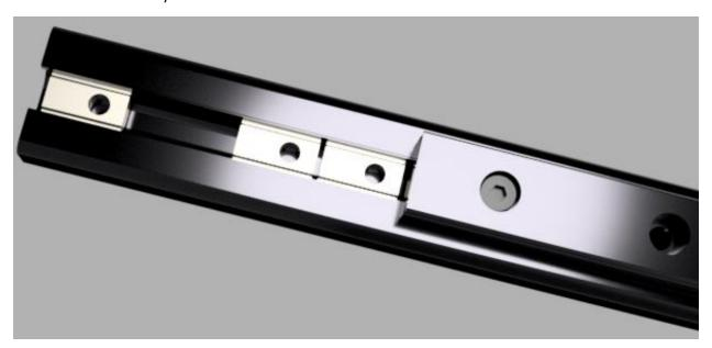
Slide the assembled Y-Axis Bracket Rear onto the X-Axis linear rail assembly and line the holes in the roll-in nuts to the holes in the printed assembly.
