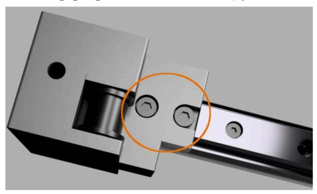
Install a ISO7380\_M4\_30mm\_BHHS into the location shown below and fully tighten.
