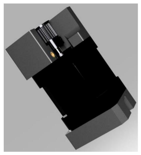
Place Print\_XY-Axis\_Motor\_Bracket\_Front\_Part01 onto the NEMA 17 motor assembly as shown and secure the printed parts to the motor with three DIN912\_M3\_45mm\_SHCS fully tightening.
