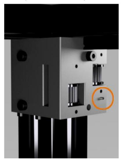
Install the printed part on the corner bracket as shown.
