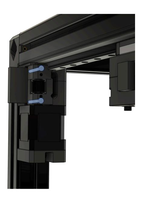
Remove the printed pre-tensioning tool. Locate Print\_XY-Axis\_Motor\_Bracket\_Rear\_Part01 and install a M3\_4.6x4mm\_Heat\_Set\_Insert in the position shown below.
