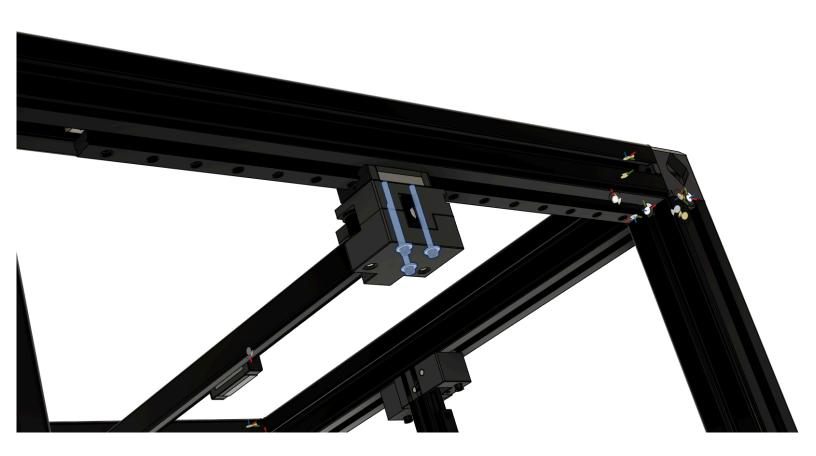
Remove the blue painters tape from the MGN-12 linear rail cartridge of the rear Y-Axis rail (if previously installed) and line it up to the rear Y-Axis bracket of the X-Gantry. Secure the bracket to the gantry with three M3 Fender Washers and three DIN912\_M3\_40mm\_SHCS.
