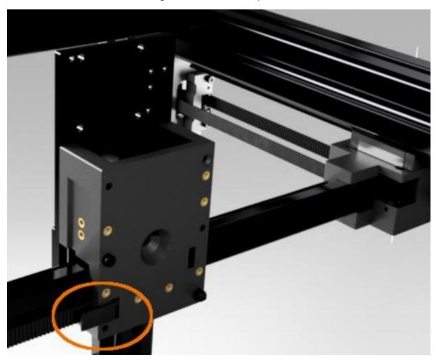
Attach a Print\_XY\_Belt\_Tightening\_Tool\_(1.52mm) to the end of XY belt.
