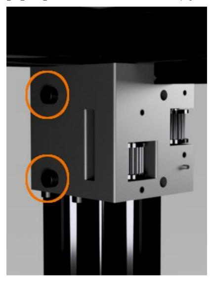
Install a DIN912\_M4\_25mm\_SHCS into the location shown below and fully tighten.
