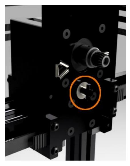
Locate a T-Lock\_Shim. These parts are extremely small, be careful not to lose them during installation. Slide one shim onto the end of the T-Lock shaft. Be certain to push the shim past the groove.
