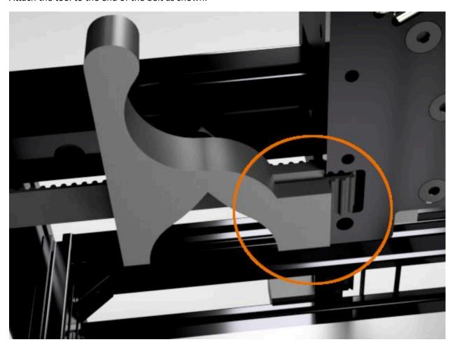
Locate CNC\_Belt\_Clamp\_Left and loosely secure with ISO7380\_M3\_8mm\_BHHS as shown. NOTE:The Belt Clamp is oriented to keep the outside edge of clamp flush to the outside edge of X-Plate.
