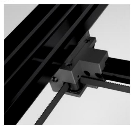
Now route the loose end of this XY belt through the rear XY motor assembly. The toothed face of the belt faces the toothed pulleys. Start by feeding the belt around the motor pulley and having the belt exit the motor assembly through the tensioner idler.
