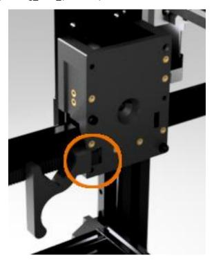
Locate Print\_BeltClamp\_Right\_Front and loosely secure with a DIN912\_M3\_10mm\_SHCS. Note:Orient this printed part so the edge of the printed clamp is flush with the front edge of the X-Bracket.
