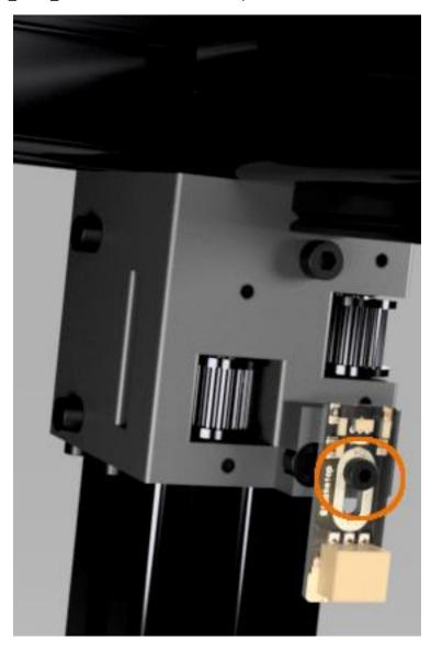
Return to Print\_XY-Axis\_Belt\_Corner\_Bracket\_Rear\_Bottom and install one of the idler pulley assemblies as shown below.
