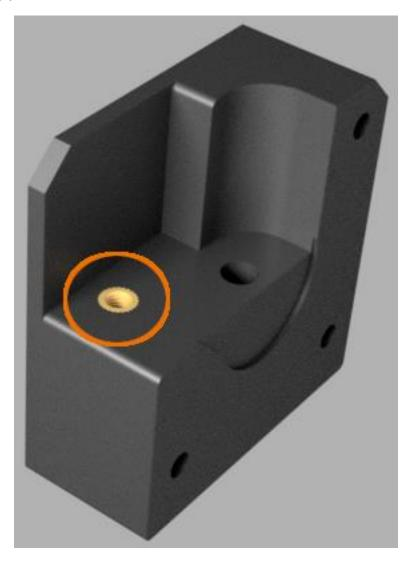
$Locate\ Print\_XY-Axis\_Motor\_Bracket\_Front\_Part02\_CE\ and\ install\ a\ M3\_4.6x4mm\_Heat\_Set\_Insert\ into\ the\ location\ shown\ below.$
