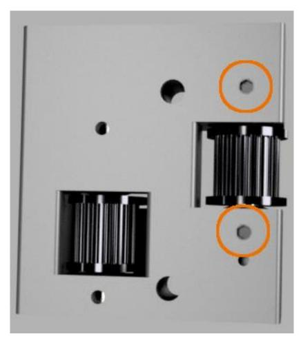
Remove the hand vise and the printed installation tools. Press one printed installation tool into the top and bottom of the corner bracket assembly covering the idler pulley assembly shown below.
