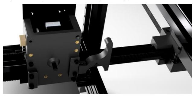
Loosen the two screws in the printed belt clamp and pull the belt with the belt pulling tool. Each tooth pulled past the edge of the printed belt clamp will gain 2mm of adjustment for the XY belt tensioner. Exposing four and a half teeth will restore the full range of the XY tensioner (8.5mm). When you have finished removing the extra slack from the XY belt, fully tighten the two screws in the printed belt clamp and remove the printed belt pulling tool.
