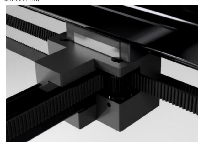
Route the loose end of the belt through left rear slot on the printed X-Bracket as shown.
