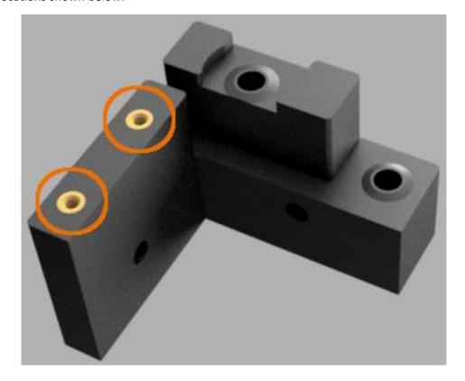
Return to Print\_XY-Axis\_Belt\_Corner\_Bracket\_Rear\_Top and install two M3\_4.6x4mm\_Heat\_Set\_Insert into the locations shown below.
