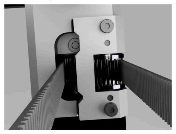
The toothed belt should only come in contact with the toothed pulleys. It should not rub or touch any other part of the machine. Verify that belt is going through tensioner housing and not around the tensioner housing.
