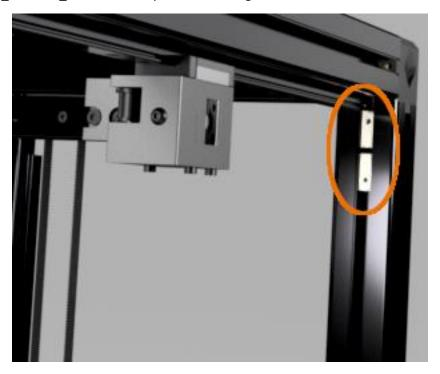
Install an additional two Tnut\_40Series\_M4 into the other inside corner of same extrusion.
