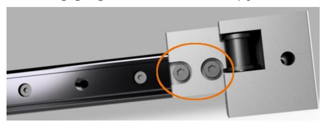
Install a ISO7380\_M4\_30mm\_BHHS into the location shown below and fully tighten.
