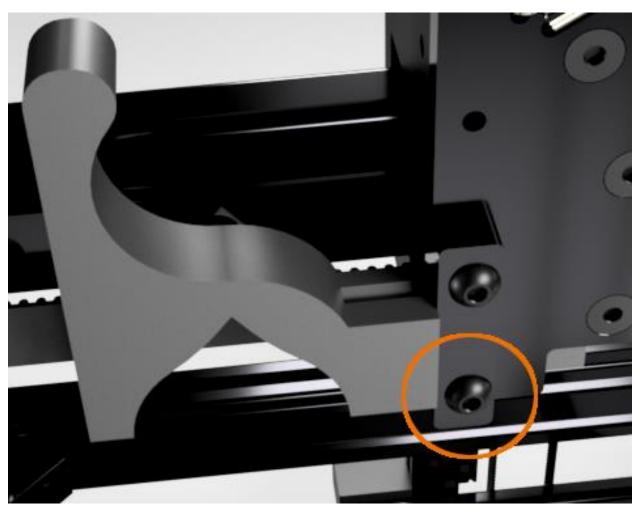
$Loosely\ install\ a\ DIN985\_M3\_Nylon\_Lock\_Washer\ onto\ the\ M3x45\ screw\ as\ shown.$
