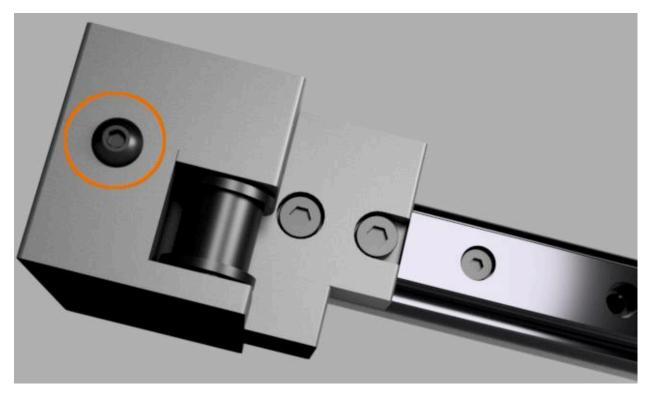
Install one of the assembled smooth idler pulleys into Print\_Y-Axis\_Bracket\_Front\_Bottom\_(1.52mm) as shown below.
