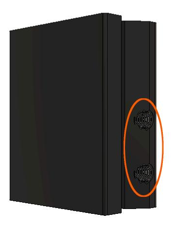
Tap M3 threads into the two holes in Printed Belt Tensioner Left Part 02 as shown below.
