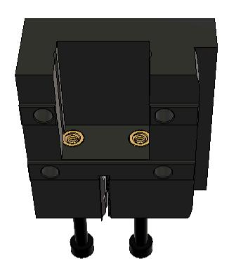
When both M4 Heat Set Inserts are cool, remove both M4x30 SHCS. Install an M3 Tap into your Hand Tap and proceed to tap M3 threads into the two holes in Printed Belt Tensioner Right Part 01 as shown below.
