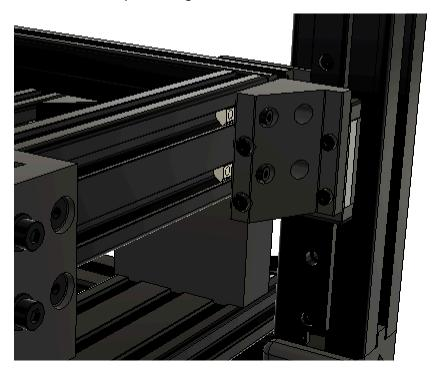
Repeat this process to secure the Z-Axis Bracket Rear to the left rear MGN12 cartridge using two additional M3x10 SHCS and two M3x35 SHCS.
