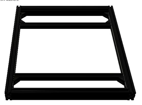
These 2020 extrusions will be the supports for your Heated Bed. The Printed Bed Frame Alignment Jigs will set these 2020 extrusions at the proper locations. To determine the proper positions of the 2020 extrusions for your bed, install the two Printed Bed Frame Alignment Jigs (56mm) on the underside of the bed frame at the right side. Move the rightmost 2020 extrusion until it lines up properly in the slots of the alignment jig.
