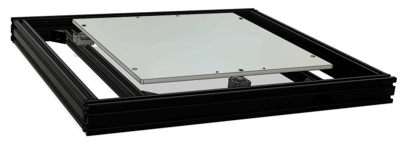
Orient the bed frame with the right side facing you and place four M4 Slot 6 roll-in nuts into the 373mm 2040 extrusion as show below.
