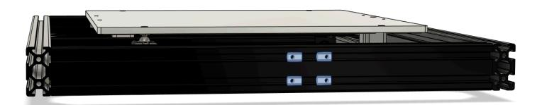
Place the assembled Printed Z-Axis Belt Tensioner Left Part 01 onto the 373mm 2040 extrusion so the holes in the printed part line up with the holes in the M4 Slot 6 roll-in nuts. You may have to move one or more of the M4 Slot 6 roll-in nuts for proper alignment. Loosely secure the printed parts to the 373mm 2040 extrusion using four M4x25 FHHS.
