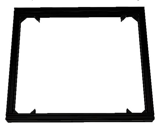
Place a 2020 extrusion of 373mm in front of you. Install two M4 Slot 6 roll-in nuts as shown.
