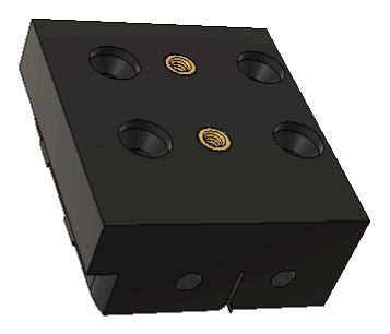
Install two M4 Heat Set Inserts into the Printed Belt Tensioner Right Part 01. You will need to hold the Soldering Iron at an angle to install the heat set inserts into this area (to prevent the Soldering Iron from melting the sides of the printed part). It is helpful to have an M4x40 SHCS inserted through the bottom of the printed part and partially screwed into the M4 heat set insert. Set up the process as shown below.
