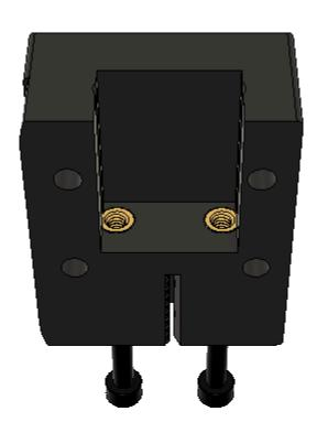
When both M4 Heat Set Inserts are cool, remove both M4x30 SHCS. Set up Printed Belt Tensioner Left Part 01 with two M4 Heat Set Inserts and two M4x30 SHCS inserted through bottom of printed part and partially threaded into M4 Heat Set Inserts.
