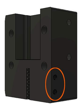
Tap M3 threads into the two holes in Printed Belt Tensioner Left Part 01 as shown below.
