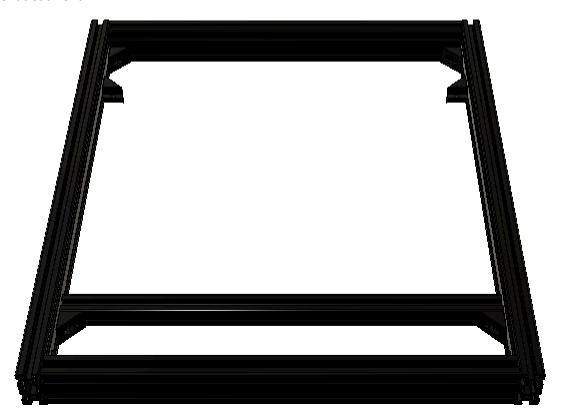
Repeat these steps with the remaining assembled 373mm 2020 extrusion using two M4x8 BHHS and two M4 washers.
