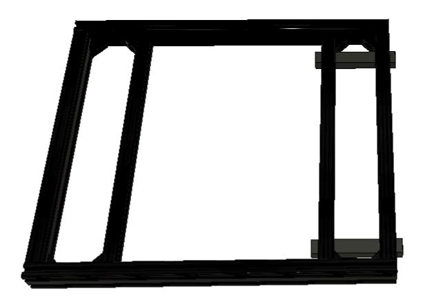
Install the Printed Bed Frame Alignment Jigs (63.5mm) on the underside of the bed frame at the left side. Move the leftmost 2020 extrusion until it lines up properly in the slots of the alignment jig.
