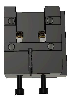
Now install the M4 Heat Set Inserts into the printed part with the Soldering Iron angled to prevent unwanted melting of the printed part. After one insert is pressed in, use the attached M4x30 SHCS to properly align the M4 Heat Set Insert until it cools. Repeat for the other M4 Heat Set Insert.
