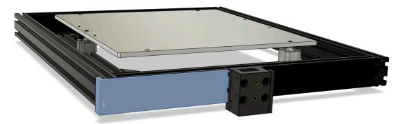
Remove the printed installation tool. Place an M4x6 SHCS through a thick M4 fender washer and loosely install into the right face of the right Z-Axis Belt Tensioner Assembly. Repeat for the other hole with another M4x6 SHCS and thick M4 fender washer.
