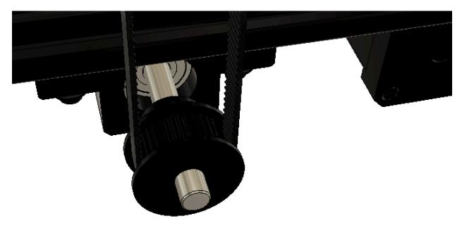
The belt routes by this guide on the rear side of the Belt Tensioner.
