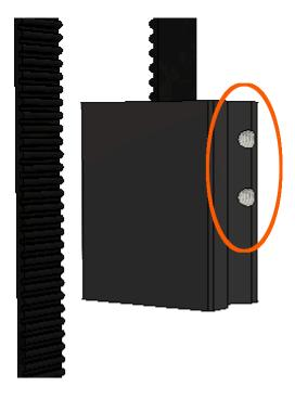
Slide Print Z-Axis Belt Tensioner Left Part 02 into Print Z-Axis Belt Tensioner Left Part 01 and loosely secure with two M4x40 SHCS each going through an M4 washer as shown below. Equally turn each M4x40 SHCS to remove slack in the belt but not enough to cause the bed to start lifting off of the printed Bed Frame Alignment Blocks. We are not tensioning the belt at this point.
