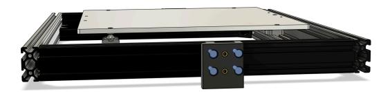
Place the Printed Z-Axis Belt Tensioner Installation Tool at the left front corner of the bed frame as shown. Move the left Z-Axis Belt Tensioner assembly so it is flush to the printed installation tool and the printed installation tool is flush to the corner of the bed frame. When properly aligned fully tighten all the M4x25 FHHS in the left Z-Axis Belt Tensioner assembly.
