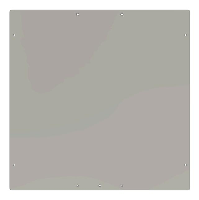
Thoroughly clean the surface of the bed using isopropyl alcohol or acetone until a clean paper towel wipe shows no transferred dirt/machining oils. It is important to follow this with a microfiber cloth wipe to remove any lint left behind.
