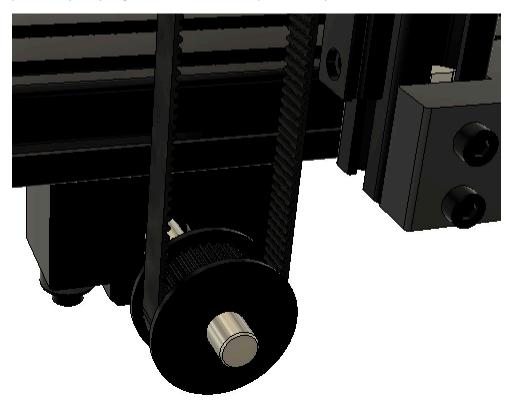
Feed the right Z-Axis Belt through the belt guide slot of the right Z-Axis Belt Tensioner Block as shown.
