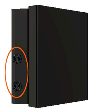
Insert one end of a GT2 Z-Axis Belt into the profile of Printed Z-Axis Belt Tensioner Part 01 as shown below.
