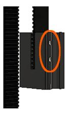
Slide Print Z-Axis Belt Tensioner Right Part 02 into Print Z-Axis Belt Tensioner Right Part 01 and loosely secure with two M4x40 SHCS each going through an M4 washer as shown below. Equally turn each M4x40 SHCS to remove slack in the belt but not enough to cause the bed to start lifting off of the printed Bed Frame Alignment Blocks.
