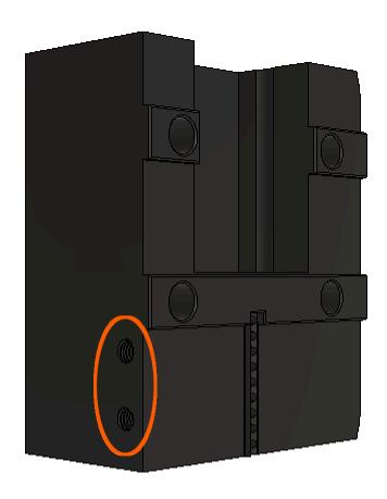
Tap M3 threads into the two holes in Printed Belt Tensioner Right Part 02 as shown below.
