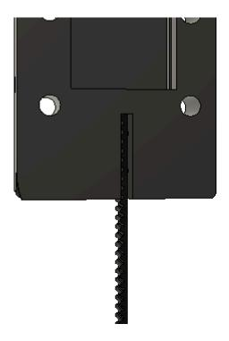
Install the two M3x6mm Set Screws into the holes you threaded earlier in Printed Z-Axis Belt Tensioner Part 01 and tighten until each Set Screw is snug against the installed GT2 Belt.
