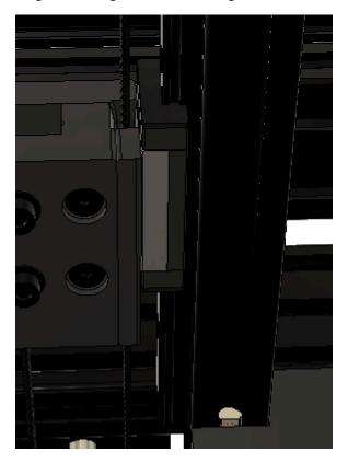
Similar to the left side of the machine, the belt feeds through one side of the Z-Axis Belt Idler assembly curves up and then around the idler pulleys then back down through the other side. It may help to bend or preform the end of the Z-Axis belt to help facilitate this routing process.
