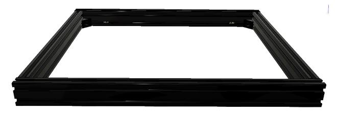
Repeat this for the front 470.5mm 2040 extrusion with two additional M4 Slot 6 roll-in nuts. Place a 2020 Corner bracket over each installed M4 Slot 6 roll-in nut and align with the threaded hole in the M4 Slot 6 roll-in nut. Loosely secure each 2020 Corner Bracket with an M4x8 BHHS through an M4 washer.
