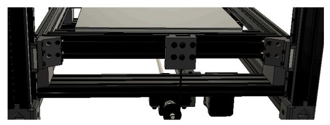
Remove the two printed Bed Frame Alignment Tools.
