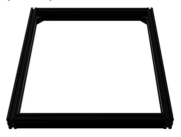
Using a carpenters square, check that each outside corner of the bed frame is 90 degrees and the 373mm extrusion is flush with the 470.5mm extrusion. Fully tighten the M4x8 BHHS as you move from corner to corner. Also measure the outermost opposing corners of the bed frame and check that the distance between them is 623.419mm. (Whatever value you manage to measure needs to be the same when you measure the other two opposing corners).
