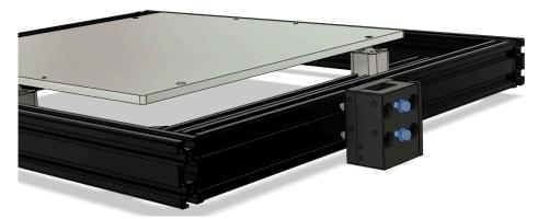
Turn the bed frame around so the left side is facing you and place four M4 Slot 6 roll-in nuts into the 373mm 2040 extrusion as show below.
