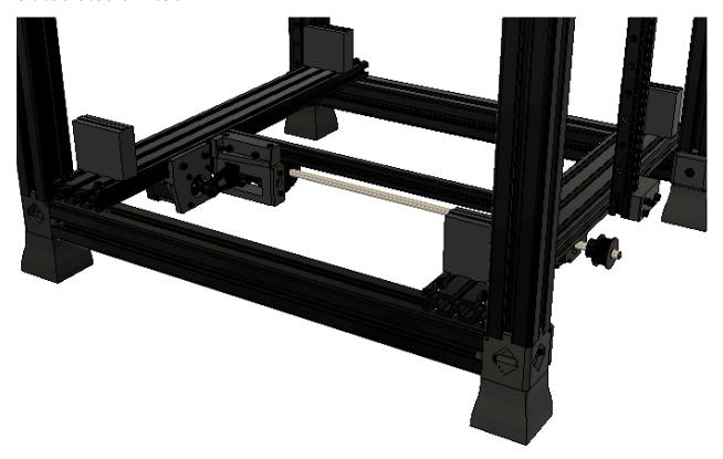
Place the assembled bed frame on top of the printed Bed Frame Alignment Blocks. The bed frame should be stable and flush to the printed alignment blocks at each corner. If your bed frame is skewed so that one corner has some space between the alignment block and associated extrusion, then loosen the SHCS in the a outer 20240 corner brackets and press the bed frame extrusions firmly toward the alignment blocks until they are flush at each corner and re-tighten all SHCS.
