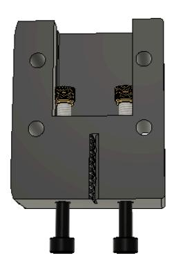
Now install the M4 Heat Set Inserts into the printed part with the Soldering Iron angled to prevent unwanted melting of the printed part. After one insert is pressed in, use the attached M4x30 SHCS to properly align the M4 Heat Set Insert until it cools. Repeat for the other M4 Heat Set Insert.
