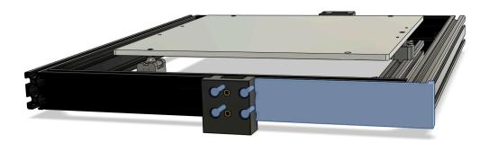
Remove the printed Installation Tool.
