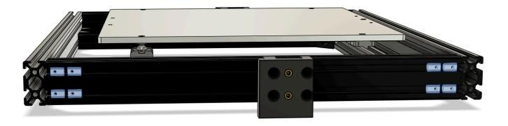
Place the Print Z-Axis Bracket Front on the 373mm 2040 extrusion at the front end (right in perspective of picture) and line up the holes in the printed part with the threaded holes of the M3 Slot 6 roll-in nuts. You may need to move one or more M3 Slot 6 roll-in nuts for proper alignment. Loosely secure the Print Z-Axis Bracket Font to the 373mm 2040 extrusion with four M3x14 SHCS.
