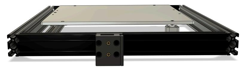
Place the Printed Z-Axis Belt Tensioner Installation Tool at the right front corner of the bed frame as shown. Move the right Z-Axis Belt Tensioner assembly so it is flush to the printed installation tool and the printed installation tool is flush to the corner of the bed frame. When properly aligned fully tighten all the M4x35 FHHS in the right Z-Axis Belt Tensioner assembly.
