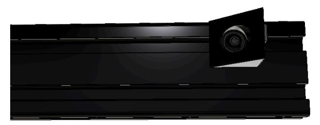
Repeat these steps at the other end of the same 2040 extrusion using another M4 Slot 6 roll-in nut, 2020 Corner Bracket, M4x8 BHHS, and M4 washer.
