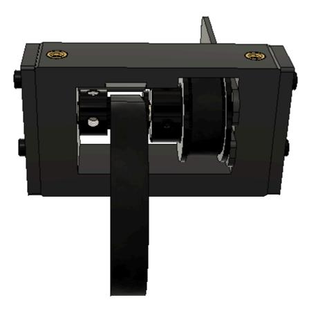
Rotate the assembly and insert the printed Pulley Reduction 16t Installation Tool between the hub of the 40t pulley and the hub of the 16t pulley.
