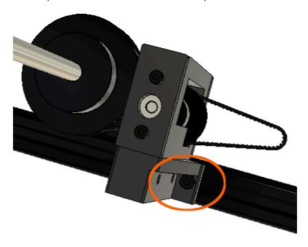
Hold the assembled 1020 extrusion against the Pulley Reduction Assembly and move the M4 Slot 6 roll-in nuts until they line up with the holes in the Pulley Reduction Assembly.
