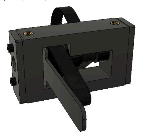
From the rear side of the Pulley Reduction assembly, secure the 40t pulley to the 5x70mm shaft. Apply medium strength thread locker to two M4x6mm Set Screws. Hold the 40t pulley tight to the left of the Pulley Reduction Assembly using the printed tool to set the proper clearance. Tighten the M4x6mm set screws into the hub of the 40t pulley completely. You may need to rotate the 40t pulley to access one or both of the set screw holes in the hub.
