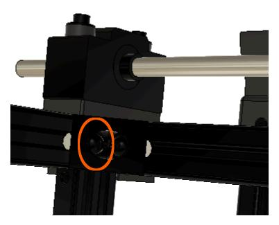
And tighten completely the M4x14mm SHCS of the Pulley Reduction Assembly.
