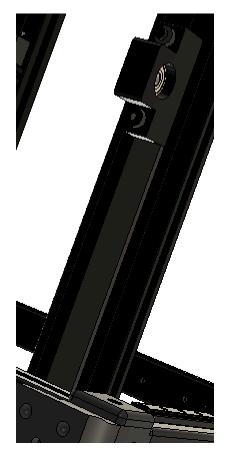
Remove the printed EF10 Installation Tool. Locate the printed Z-Axis 80t Pulley Installation tool. Slide the 8x520mm linear shaft into the printed tool until it is flush to the bottom. Install the GT2 80t pulley so the flat side of the pulley is flush with the printed tool. Coat two M5x12mm set screws with medium strength thread locker. Secure the 80t pulley to the 8x520mm linear rod with the two M5x12mm set screws. Tighten the two M5x12mm set screws completely.
