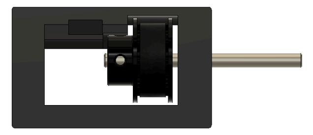
Locate the GT2 94tooth 9x188 loop belt and place it around a GT2 16t pulley with 5mm bore.
