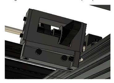
At the other end of the 1020 extrusion, secure the 2020 Corner Bracket to the right 2060 extrusion by inserting an M4x8mm BHHS through an M4 washer, through the 2020 Corner Bracket, and into the M4 Slot 6 roll-in nut. Loosely secure the M4x8mm BHHS.
