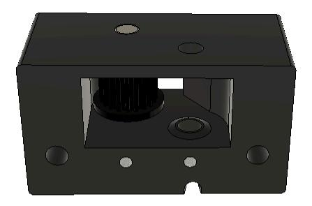
Repeat this for the other location with another GT2 20t Idler Pulley with 5mm Bore and another 5x25 Linear Shaft.
