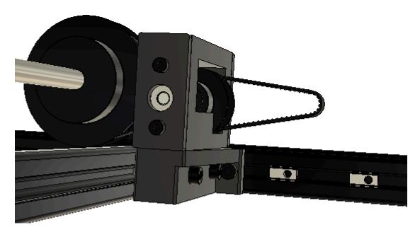
Place an M4 Slot 6 roll-in nut into the bottom of the left 2060 extrusion as shown.
