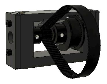
Rotate the assembly and insert the printed Pulley Reduction 40t Installation Tool between the flat face of the 40t pulley and the printed Pulley Reduction Part 02.
