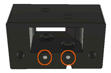
Place an M4 heat set insert into the hole as shown.
