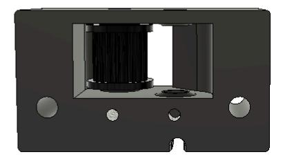
Press a 5x25mm Linear Shaft through the hole in the top of the printed part and fully through the Idler Pulley until the end of the linear shaft is flush with the rear (top in perspective of picture) of the printed part. Use the hand vise or arbor press if the linear shaft seems difficult to press in by hand.
