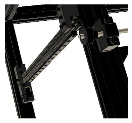
Place the printed Z-Axis Idler Pulley Installation Tool with the ribbed side toward the underside of the 420mm 4040 extrusion. Slide the Z-Axis Idler Pulley assembly until it is flush with the printed Installation Tool and the printed tool is flush to the 395mm 4040 extrusion. Fully tighten the two M4x35 SHCS.
