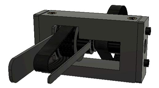
From the rear side of the Pulley Reduction assembly, secure the 16t pulley to the 5x70mm shaft. Apply medium strength thread locker to two M4x4mm Set Screws. Hold the 16t pulley tight to the left of the Pulley Reduction Assembly using the printed tool to set the proper clearance. Tighten the M4x4mm set screws into the hub of the 16t pulley completely. You may need to rotate the 16t pulley to access one or both of the set screw holes in the hub.
