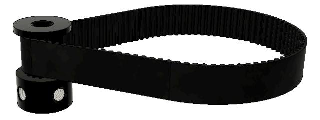
Insert a flanged 5x10x4 bearing into the pocket on the right face of the printed part. Insert the GT2 16t pulley into the printed part with the hub facing the hub of the 40t pulley. Continue to press the 5x70mm linear shaft through the 16t pulley, through the printed part, and through the 5x10x4 flanged bearing. Squeeze each end of the 5x70mm linear shaft to center it into the printed part.
