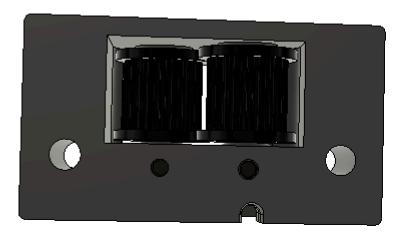
Press a 4x9x4 Bearing into printed Z-Axis Tackle Roller.
