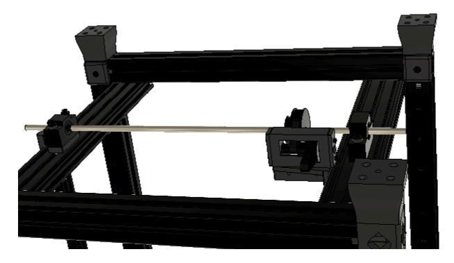
Place the ribs of the printed Z-Axis EK8 Installation Tool into the center slot of the 2060 rail between the EK8 Bearing and the front 470mm 4040 extrusion. Slide the EK8 Bearing assembly until it is flush with the printed installation tool and the printed installation tool is flush to the 470mm 4040 extrusion. Fully tighten all the M4x45 SHCS.
