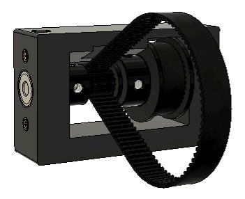
Locate the two printed Pulley Reduction Part 03. You will notice that one face of these printed parts has a recess. Install one of these printed parts onto the right of the Pulley Reduction assembly with the recess facing the flanged 5x10x4 bearing, then secure with two M3x8mm SHCS. Repeat this with the other printed part and two more M3x8mm SHCS on the left end of the Pulley Reduction Assembly.
