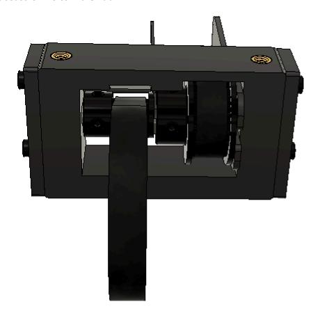
Remove the printed Pulley Reduction Installation Tools. Place the printed Pulley Reduction Part 01 on top of the Pulley Reduction Assembly and secure with two M4x20 SHCS.
