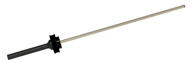
Remove the printed tool from the linear shaft. If you find it difficult to remove the printed tool, you can install a M3 heat set insert into the bottom of the printed tool while it is still attached to the linear shaft,
