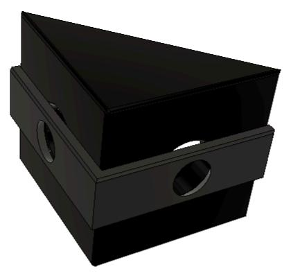
Now insert a Print\_2020\_Corner\_Bracket\_Lock\_Part\_02\_CE through one of the holes of the 2020 Corner Bracket until it is flush with the bracket and locked into the printed Part 01.
