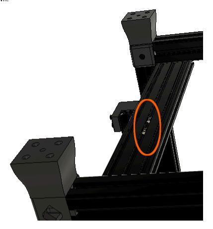
Place the printed part EK8 Spacer on top of the 2060 extrusion and align the holes of the M4 Slot 6 roll-in nuts with the holes in the printed part.
