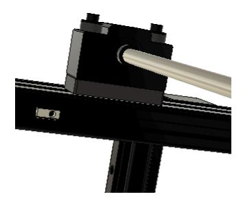
Place the assembled 1020 extrusion against the Pulley Reduction Assembly again. Secure the Pulley Reduction Assembly to the 1020 extrusion with two M4x22mm SHCS. Keep the 1020 extrusion flush to the left 2060 extrusion and tighten the two M4x22mm SHCS completely.
