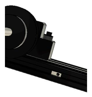
Move the Pulley Reduction Assembly back into position and insert an M4x14mm SHCS through the Pulley Reduction Assembly into the M4 Slot 6 roll-in nut. Loosely fasten the M4x14mm SHCS.
