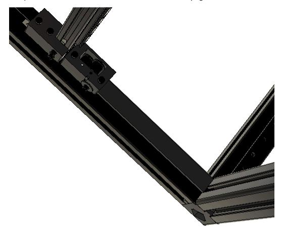
Remove the printed Installation tool. Repeat the previous steps to install the left Z-Axis Belt Pulley Idler assembly. Turn the frame upright. Congratulations, you have completed the Z-Axis Motion Assembly.
