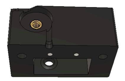
Orient the part as shown and snap a GT2 20t Idler Pulley with 5mm Bore into printed part. The upper Idler Pulley must be installed first.
