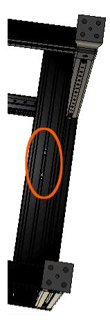
Place the EF10 Bearing on top of the left 2060 extrusion. Line up the holes in the M4 Slot 6 roll-in nuts with the mounting holes in the EF10 Bearing.
