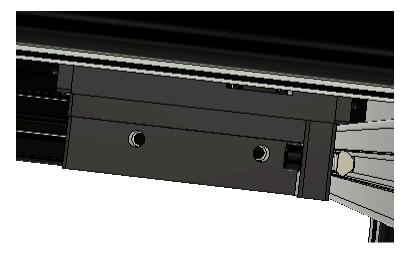
Put the assembled 1020 extrusion down. Install an M4 Slot 6 roll-in nut on the side of the right 2060 extrusion as shown.
