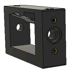
Insert a flanged 5x10x4 bearing into the pocket on the left face of the printed part.
