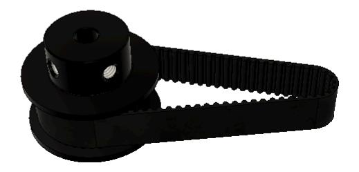
Place the GT2 40t pulley into the printed part with the hub facing toward the right (left for perspective of picture) of the printed part. The pulley can only fit into the part one way. Press the 5x70mm linear shaft through the flanged bearing, through the printed part, and through the GT2 40t pulley until it just protrudes from the hub of the pulley.
