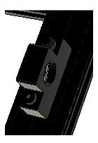
Place the ribs of the printed Z-Axis EF10 Installation Tool into the center slot of the 2060 rail between the EF10 Bearing and the front 470mm 4040 extrusion. Slide the EF10 Bearing assembly until it is flush with the printed installation tool and the printed installation tool is flush to the 470mm 4040 extrusion. Fully tighten all the M4x35 SHCS.
