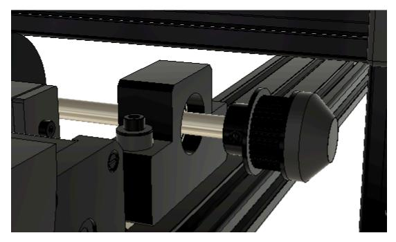
Remove the printed Installation Tool. Repeat the above steps to install the other GT2 40t Pulley with 8mm Bore on the right end of the 8x520mm linear shaft using the printed Installation Tool and two M4x4mm set screws coated in medium strength thread locker.
