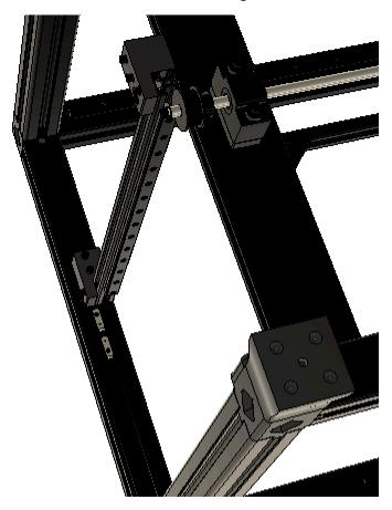
Place the right Z-Axis Belt Idler assembly on the underside of the right 420mm 4040 extrusion and align the holes of the M4 Slot 8 roll-in nuts with the holes in the assembly. Loosely attach two M4x35mm SHCS through the Z-Axis Belt Idler assembly into the M4 Slot 8 roll-in nuts.
