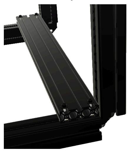
Repeat this process for the other side with the remaining 2060 extrusion, 4 M4x30 SHCS, and 4 M4 fender washers.
