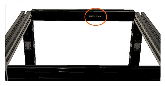
Insert two M4 Slot 6 roll-in nuts into the right side of the 482mm 2060 extrusion as shown below. The exact positions will be realized later.
