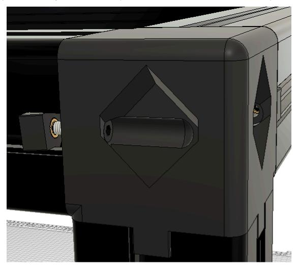
Using the angled end of your M3 hex wrench, tighten the M3x10 SHCS while pressing on the printed Corner Bracket Lock until the M3x10 SHCS pulls the printed Corner Bracket Lock flush to the printed Corner Bracket Top and is tight. Repeat the process with another M3x10 SHCS on the other face of the printed Corner Bracket Top.
