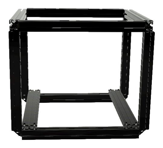
Now to verify frame is square, measure the distance between the outer faces of the lower 470mm 4040 extrusions. The distance should be 500mm at each end. Adjust if necessary while keeping the 2060 extrusions flush with the vertical 395mm 4040 extrusions. Tighten all the M4 screws of the 2060 extrusions. Note: The 2060 extrusions have a light profile and cannot handle over-tightening. Any excessive tightening into a roll-in nut will cause the nut to deform the extrusion it is housed in.
