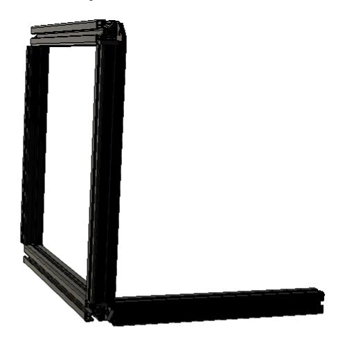
Attach another 395mm extrusion to the other lower corner bracket of the upper frame with a M8x25mm BHHS.
