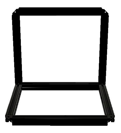
Using a carpenters square, check that the angle between the side frame and the upper frame is 90 degrees.
