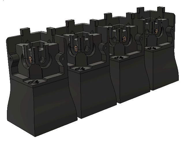
The two printed brackets to the left will attach to the Rear Left and the Front Right. The two printed brackets to the right will attach to the Front Left and Rear Right.
