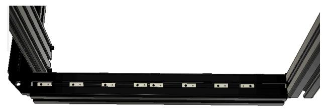
Place the MGN12 rail assembly onto the 395mm 4040 extrusion and secure it with three printed 4040 MGN12 Alignment Blocks.
