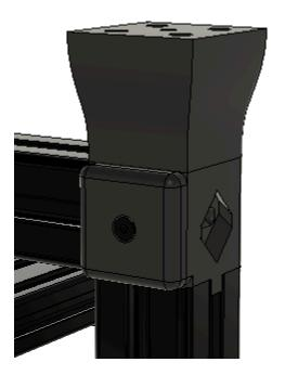
Insert an M3x10 SHCS in the recessed hole of the printed Corner Bracket Bottom on the opposite face. Fully press the screw in by hand moving the printed Corner Bracket Lock.
