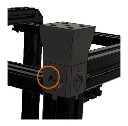
Line up the M3 heat set insert in one of the printed Corner Bracket Bottom Lock parts with the M3x10 SHCS you just installed into the printed Corner Bracket Bottom. Using the angled end of your hex wrench, tighten the M3x10 SHCS allowing the screw to pull the printed Corner Bracket Bottom Lock flush to the printed Corner Bracket Bottom. Be certain the keyed post on the printed Corner Bracket Bottom Lock is properly aligned so it goes through the Aluminum Corner Bracket.
