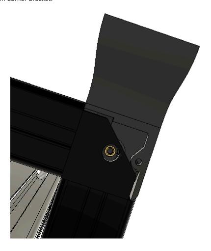
Place an M3x10 SHCS fully into the recessed pocket of the Corner Bracket Bottom.
