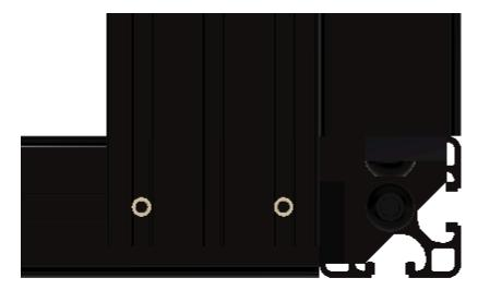
Insert a M4x30mm SHCS through a M4 fender washer and insert through one of the holes of the 2060 extrusion then fasten to the M4 Slot 8 roll-in nut. Repeat for the three other holes of the 2060 extrusion. Check that the 2060 extrusion is flush against the two 395mm 4040 extrusions.
