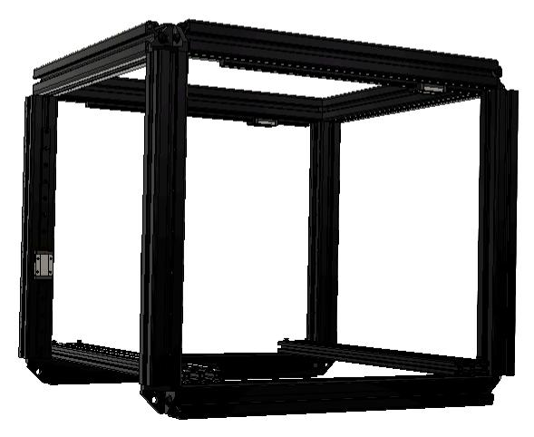
Move the frame aside and place the 2020 extrusion of 395mm in front of you. Locate the remaining 335mm MGN12 rail and remove the blue painters tape if installed in the preparation section. Be careful not to let the MGN12H carriage slide to the end or off the rail as you move it around during installation. Insert eight M3 Slot 6 roll-in nuts into the 395mm 2020 extrusion as shown. The exact positions will be realized as the MGN12 rail is secured.
