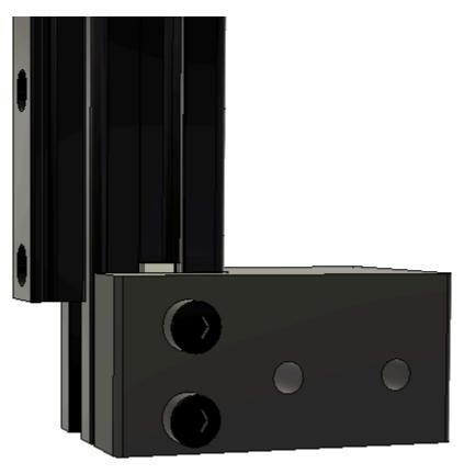
Insert two M4 Slot 6 roll-in nuts into the other end of the 395mm 2020 extrusion as shown. The exact positions will be realized later.
