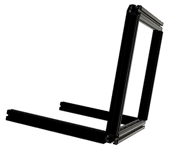
Take another 4040 extrusion of 470mm and attach a corner bracket to each end with a M8x25 BHHS.
