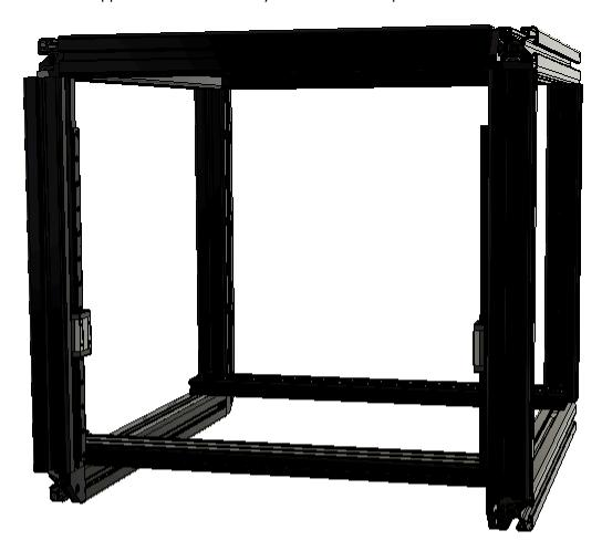
Rotate the frame so the top is facing work surface and front side facing you. Locate one of the 400mm MGN12 rails and remove the blue painters tape if installed in the preparation section. Be careful not to let the MGN12H carriage slide to the end or off the rail as you move it around during installation. Insert nine M3 Slot 8 roll-in nuts into the bottom face of the front 470mm 4040 extrusion as shown. The exact positions will be realized as the MGN12 rail is secured.
