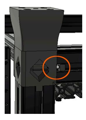
Put pressure on the printed Corner Bracket Lock as you tighten the M3x10 SHCS with the angled end of a hex wrench. As you tighten the M3x10 SHCS the printed Corner Bracket Lock will move toward the printed Corner Bracket Bottom. Continue to tighten until these printed parts are flush and tight.
