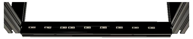
Place the MGN12 rail assembly onto the 470mm 4040 extrusion and secure it with three printed 4040 MGN12 Alignment Blocks.
