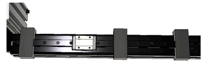
Now that all the M3x14 SHCS are loosely screwed into their proper holes, install the Print\_Z-Axis\_Left\_Linear\_Rail\_Installation\_Tool\_(10)\_CE into the Slot 8 of the 4040 extrusion. Slide the MGN12 rail so the bottom of the rail is flush to the printed Installation Tool and the printed Installation tool is flush to the 4040 Corner Bracket.
