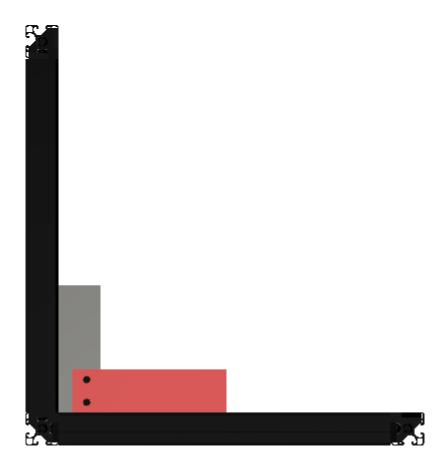
And check that the distance between opposing inside corners of side frame is 613.942mm. (Whatever value you manage to measure needs to be the same when you measure the other two opposing corners). Give these screws for the side frame a final tighten.
