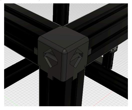
Insert an M3x10mm SHCS into the recessed hole of the printed Corner Bracket Top, then push the screw in by hand with enough force to move the printed Corner Bracket Lock until the screw is fully seated.
