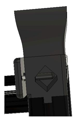
When the printed Corner Bracket Bottom Lock is flush and tight to the printed Corner Bracket Bottom, install an M4x25 FHHS through the center of the printed Corner Bracket Bottom Lock and into the printed Corner Bracket Bottom, then fully tighten.
