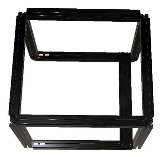
Verify the holes for the roll-in nuts are centered in the holes drilled through the 2060 extrusion. Repeat for other end.
