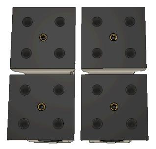
Locate and install a Print\_TPU\_Foot\_CE onto each corner foot using (4 total) M4x10mm FHHS
