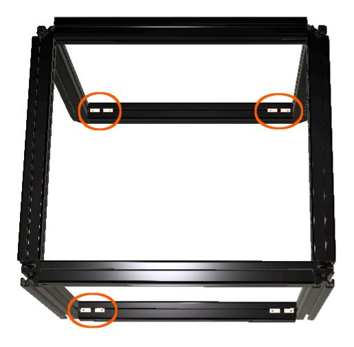
Place one 2060 extrusion on top of the two lower 470mm 4040 extrusions.
