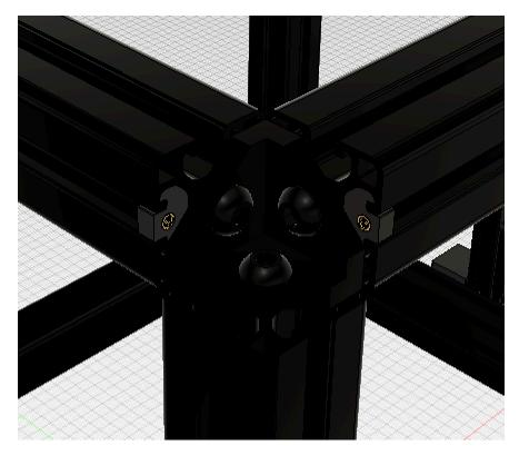
Insert a printed Corner Bracket Top as shown.
