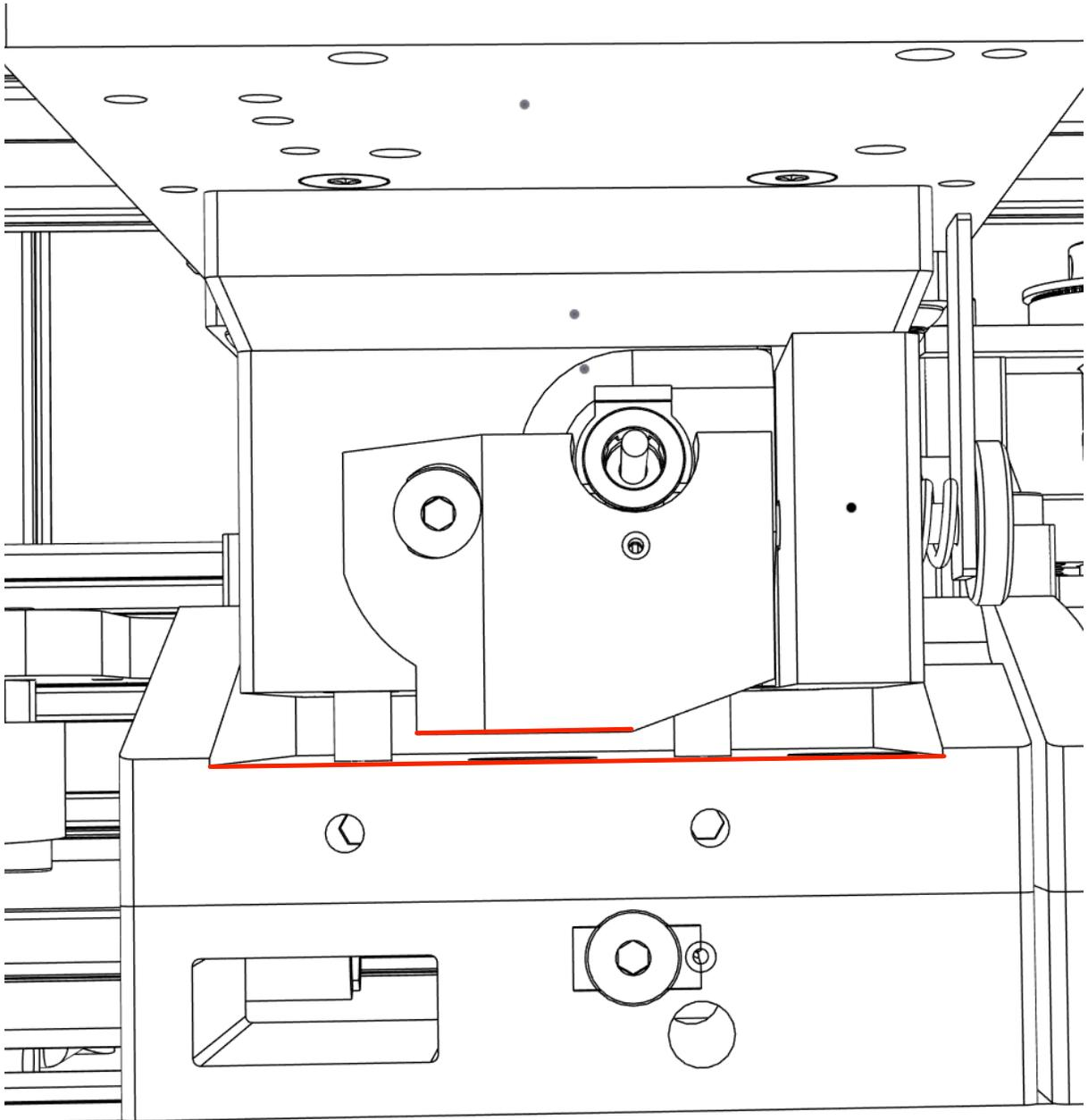
**Slowly jog the tool head in +0.1mm increments using using Duet Web Control in the Y+ direction while using your free hand to check the amount of movement allowed at each position (image below). The target value will meet the following conditions:**
