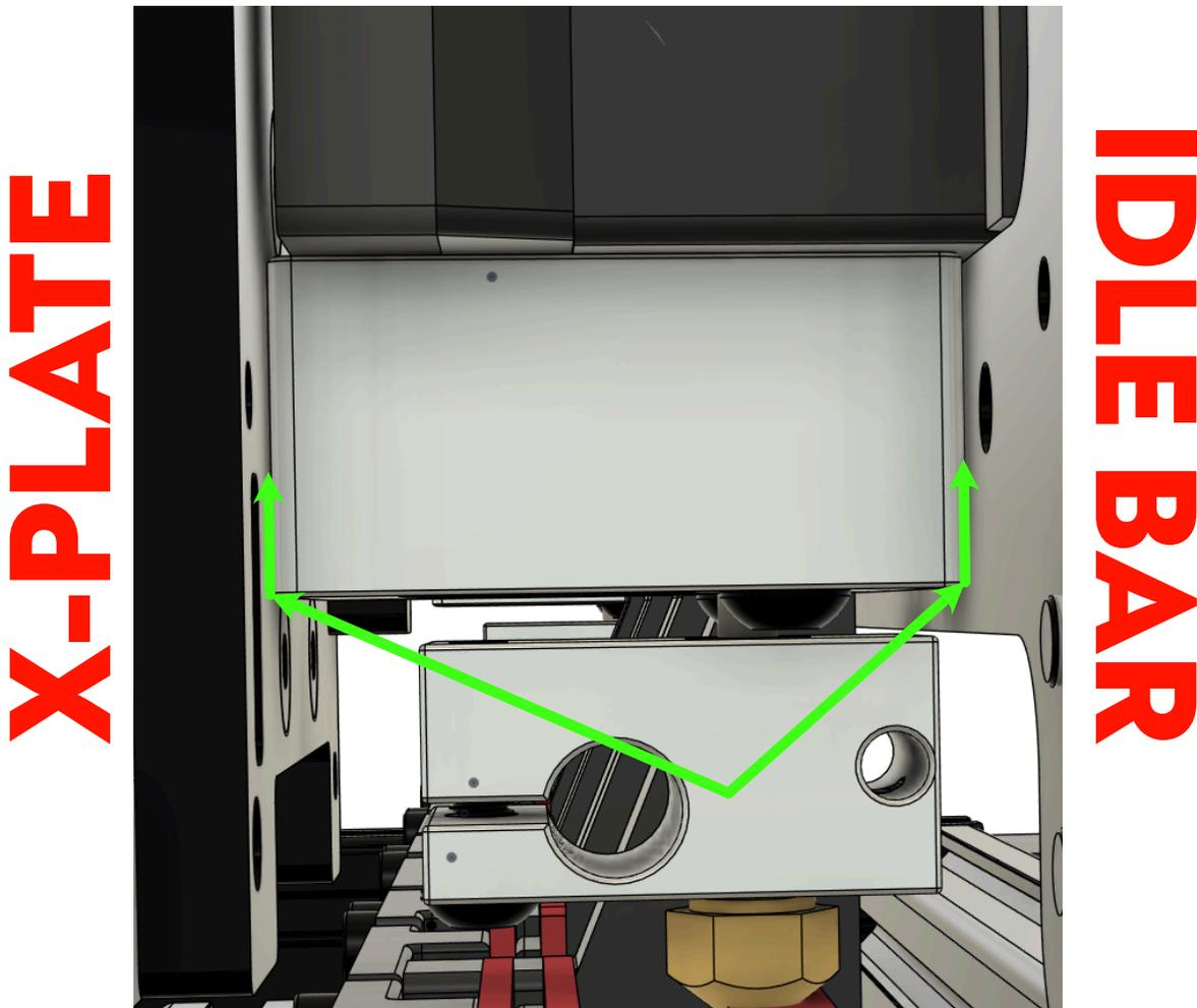
Jog the Y axis of the machine toward Y min until the extruder drive gear is clear of the now parked tools key way.
