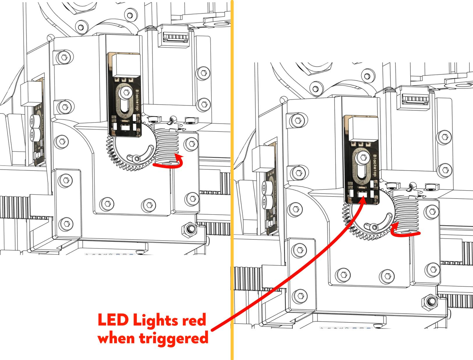
**Now rotate the worm driver gear clockwise slowly until the Blackstop LED light is triggered. At this exact position the T-lock should be horizontal.**
