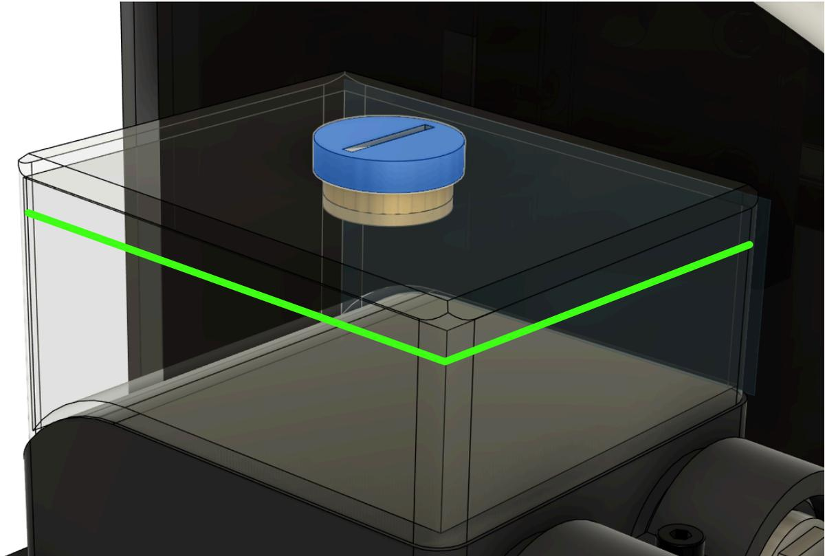
Leave the plug out for now, as multiple top ups will be needed as the system fills and purges air
