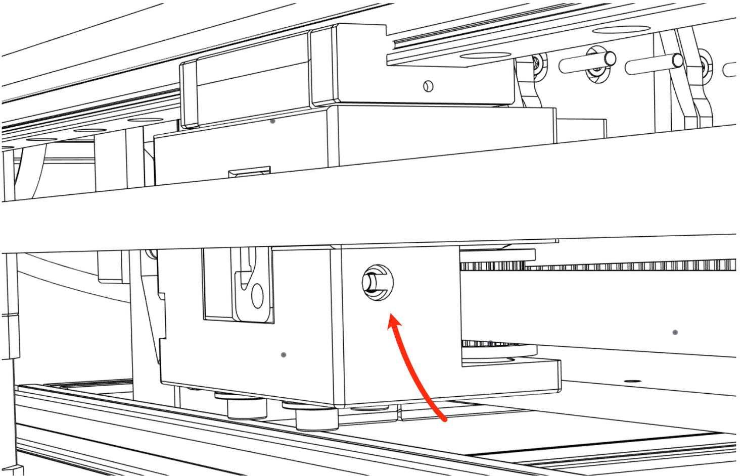
**TEST POINT:** The Y Axis End Stop Trigger is threaded in as far as it will go while also maintaining a triggered Y end stop switch and no contact between the gantry and fixed parts of the machine.
