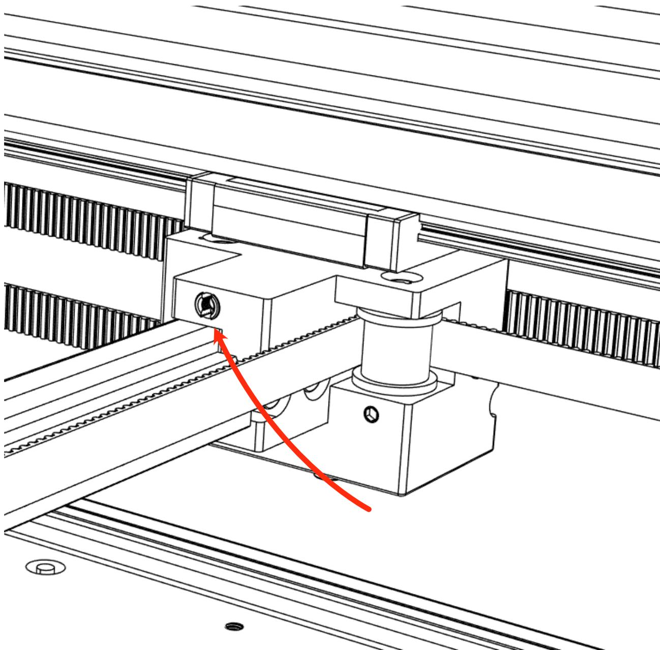
**TEST POINT:** The X Axis End Stop Trigger is threaded in as far as it will go while also maintaining a triggered X end stop switch and no contact between the gantry and fixed parts of the machine.
