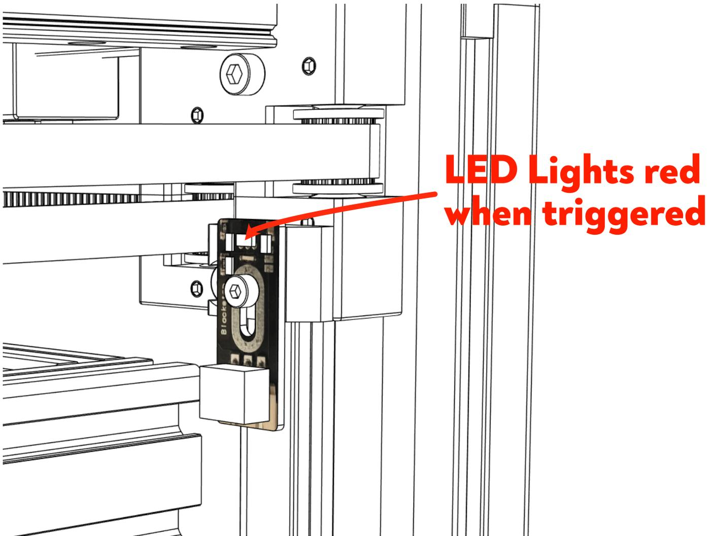
**Adjust the end stop trigger inward (deeper) slowly while checking often that the end stop DOES trigger AND there is no contact between the gantry and any other part of the machine. A fully seated trigger with no additional adjustment is okay.**
