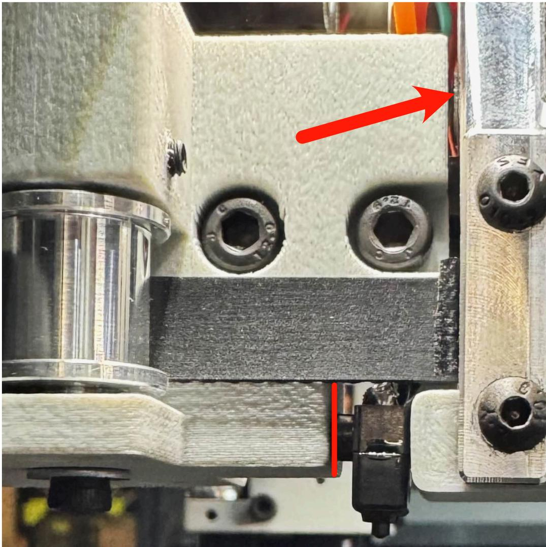
**Confirm that sufficient (though minimal) gap exists between the tool head and XY gantry at an absolute position of X308.5.**
