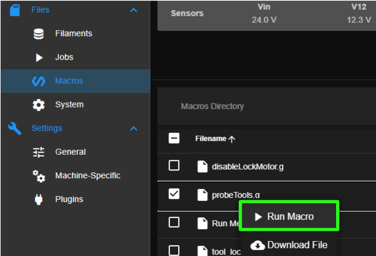
The screenshot shows the DWC interface with the 'Macros' tab selected in the left sidebar. The main area displays the 'Macros Directory' with a list of files. The file 'probeTools.g' is selected, and a context menu is open over it, with the 'Run Macro' option highlighted by a green box.
