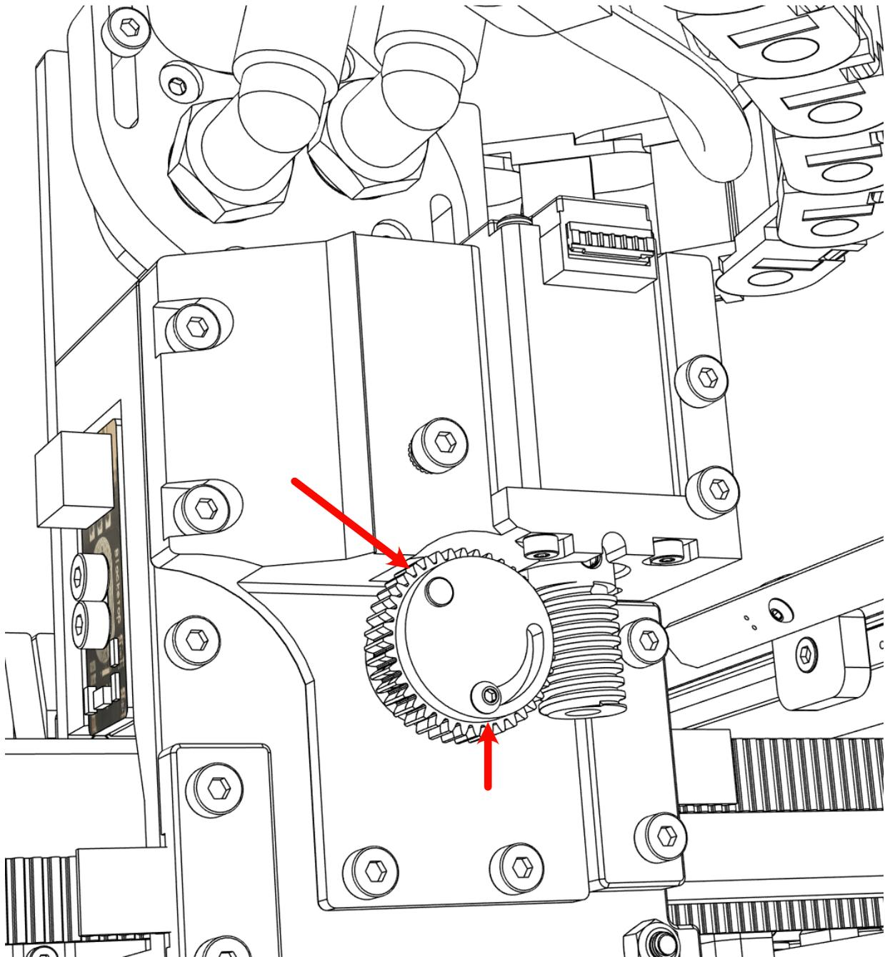
**Rotate the worm drive gear counter-clockwise by hand 2-3 full rotations. This will move the T-lock itself clockwise when viewed from the front of the X-Plate**
