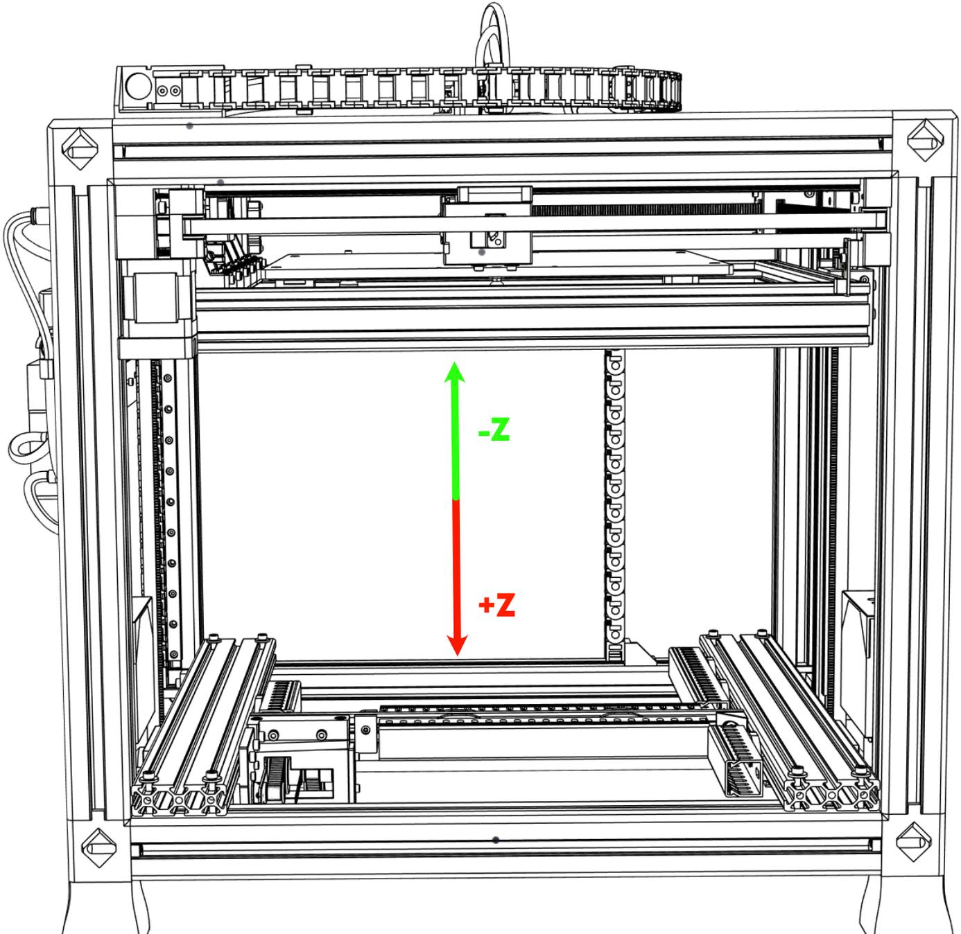
**TEST POINT:** You can now fully home the machine for the first time! Start with the bed at at least 100mm of clearance to the nozzle and the tool head near the middle of the bed. Be sure to have access to either the power switch or the emergency restart button in Duet Web Control. Here is what to expect:
