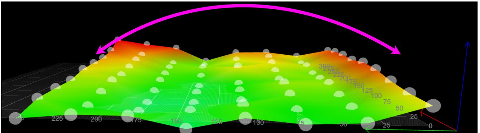
Just as noted during gantry de-racking, the printing plane's flatness should be prioritized over even belt tension (within reason)
