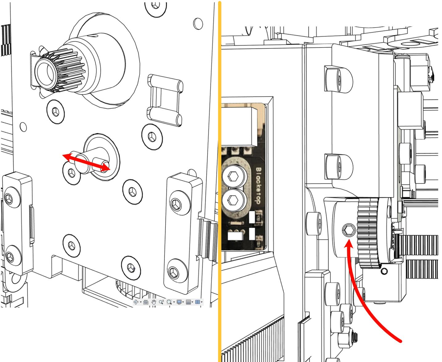
**The set screw in the 40 tooth worm driven gear should be engaged with the flat surface of the t-lock, and parallel with the X-axis.**
